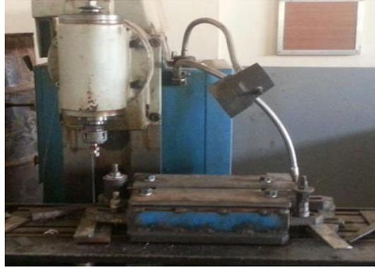
Figure 4: Classic milling machine used for BFSW process
