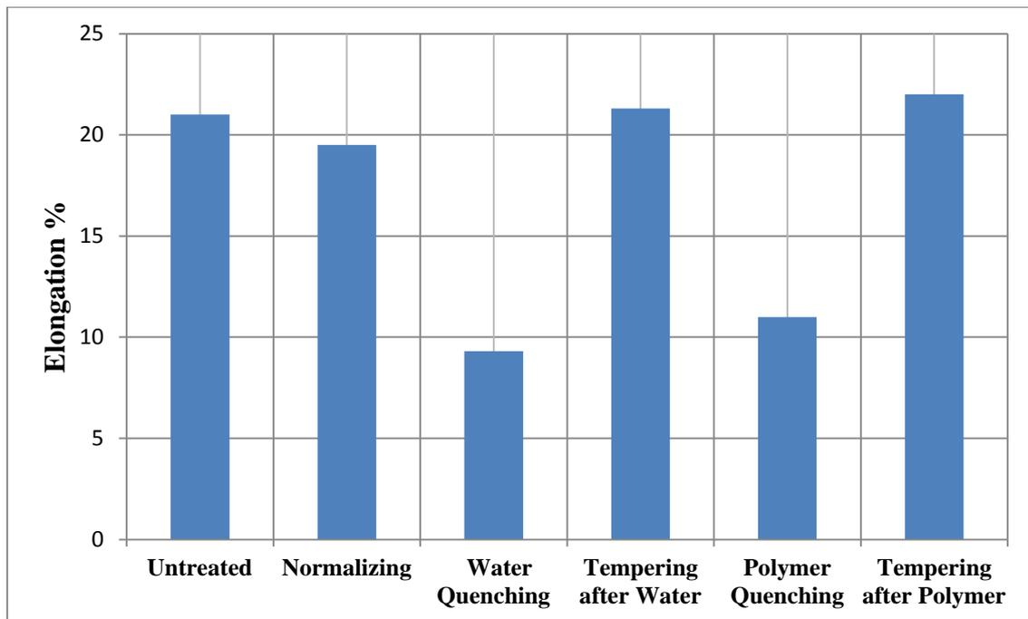
Figure 3; Elongation for untreated and heat treated samples
