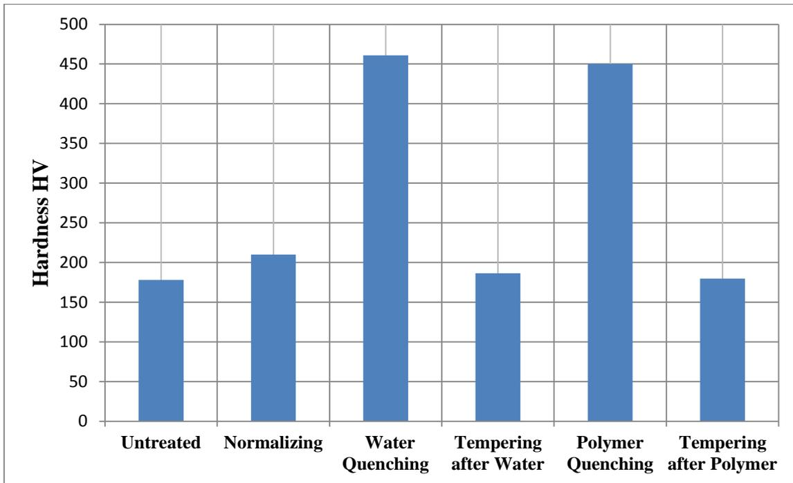
Figure 2; Hardness for untreated and heat treated samples
