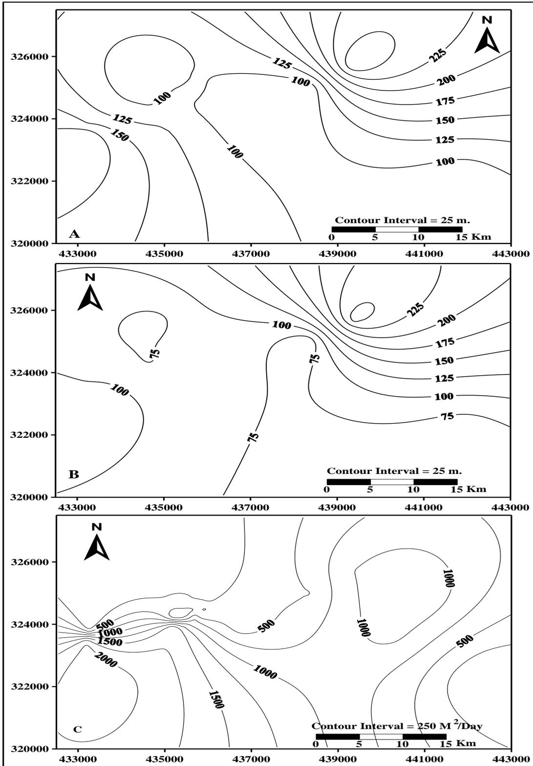
Figure (4): Depth (A), Thickness (B) and Transmissibility (C) of confined aquifer.
