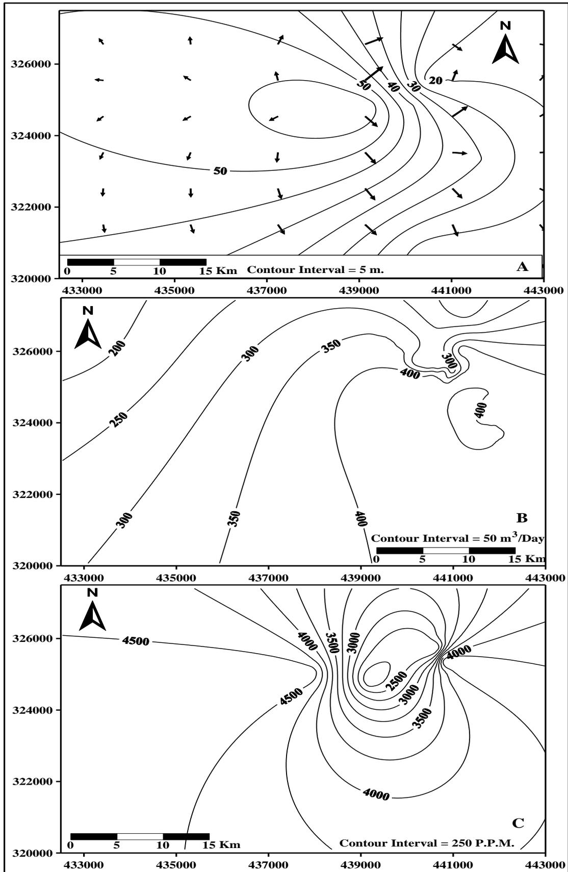
Figure (4): Water Table (A), Maximum Yield (B) and T.D.S. (C) Maps of unconfined aquifer.
