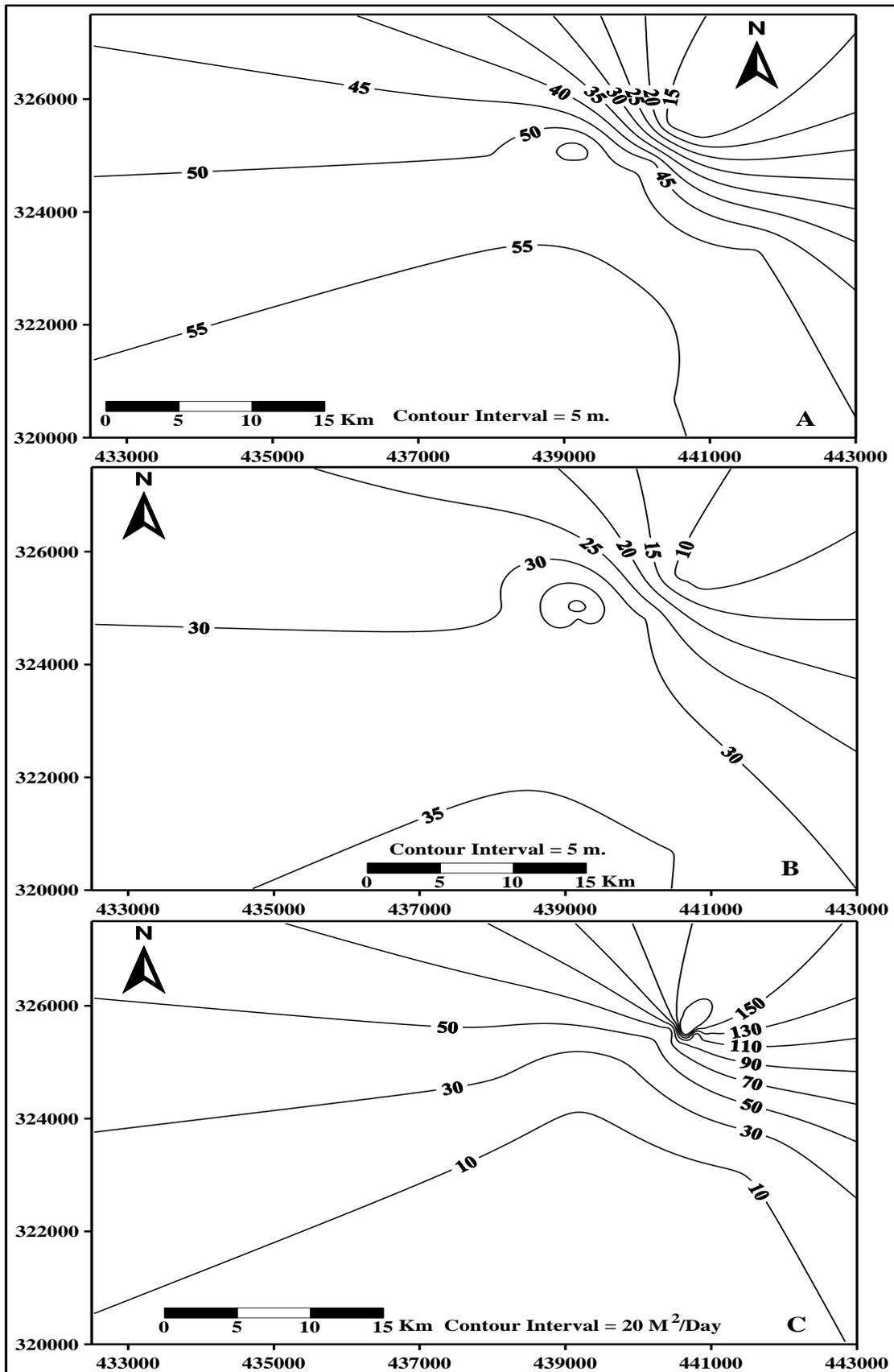
Fig (3): Depth (A), Thickness (B) and Transmissibility (C) of unconfined aquifer.
