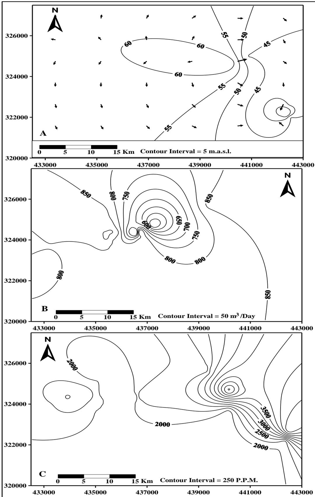
Figure (5): Piezometric levels (A), Maximum Yield (B) and T.D.S. (C) Maps of confined aquifer.
