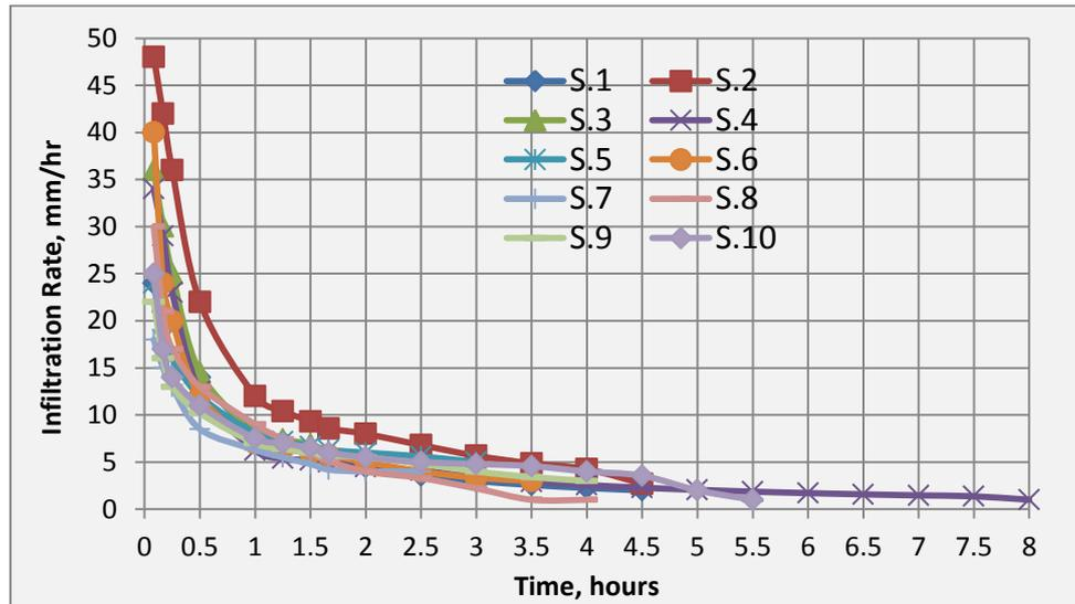
Fig.(8) Infiltrometer Results
