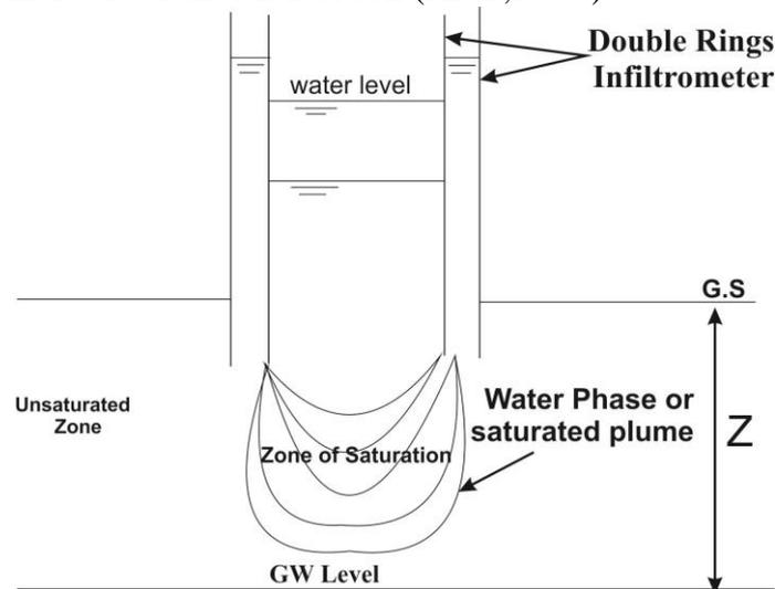
Fig.(3) Water Plume Advance in Unsaturated Zone
