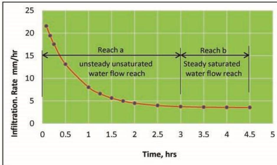
Fig.(2) Steady state saturated flow reach of arbitrary example
