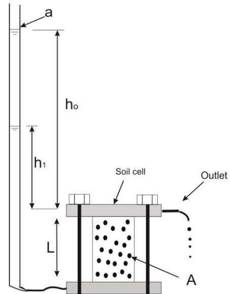
**Fig.(7)Falling Head Permeameter**
