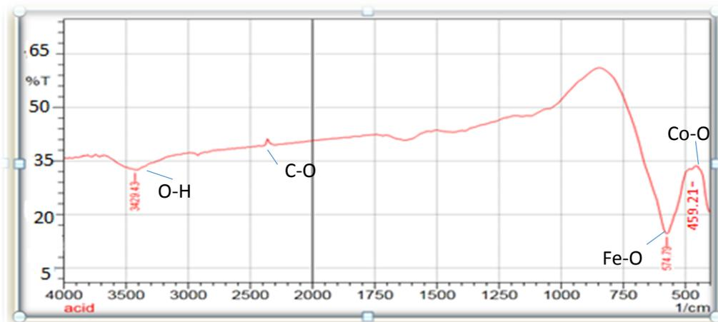
**Figure (3) FTIR for Cobalt Ferrite by Acid and Calcined at  $600^\circ\text{C}$**
