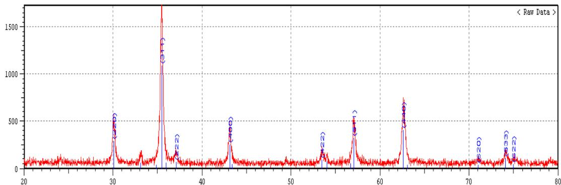
Figure (1): XRD Patterns of Cobalt Ferrite by Acid Calcined at 600 °C
