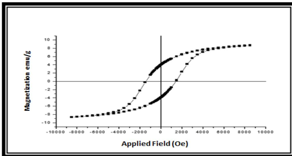
Figure (8) Hysteresis Loop of Cobalt Ferrite by Ammonium Hydroxide Calcined at 600 °C
