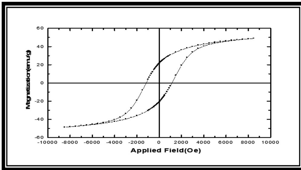
Figure (7) Hysteresis Loop of Cobalt Ferrite by Acid Calcined at 600 °C
