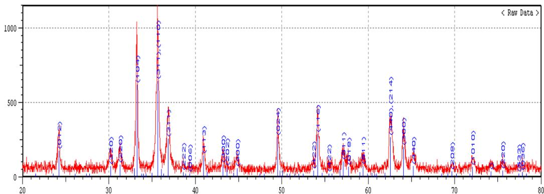
Figure (2): XRD patterns of Cobalt Ferrite by Ammonium Hydroxide Calcined at 600 °C
