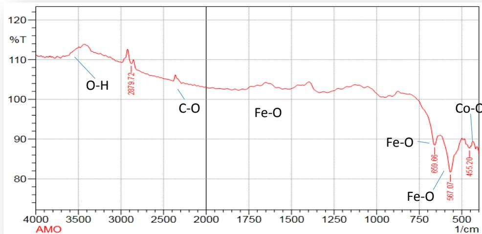
**Figure (4) FTIR for Cobalt Ferrite by Ammonium Hydroxide and Calcined at  $600^\circ\text{C}$**
