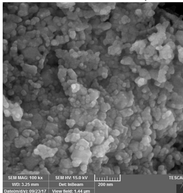
Figure (6) SEM of Cobalt Ferrite Powder by Ammonium Hydroxide Calcined at 600°C
