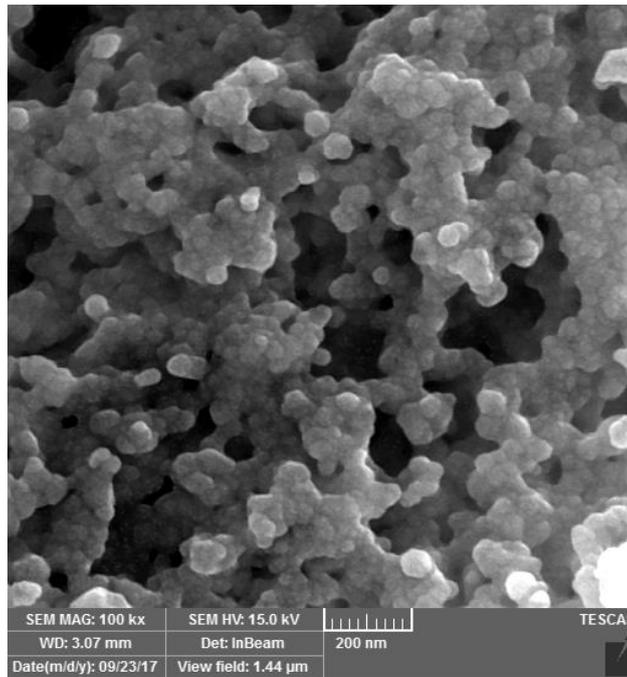
Figure (5) SEM Pattern of Cobalt Ferrite Powder by Acid Calcined at 600°C
