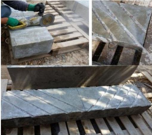
Figure (3) Groove Cutting Process
