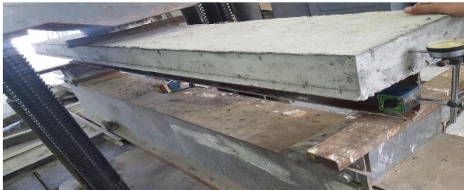
**Fig.4 Steel Concrete Composite Beam Specimen under Test**
