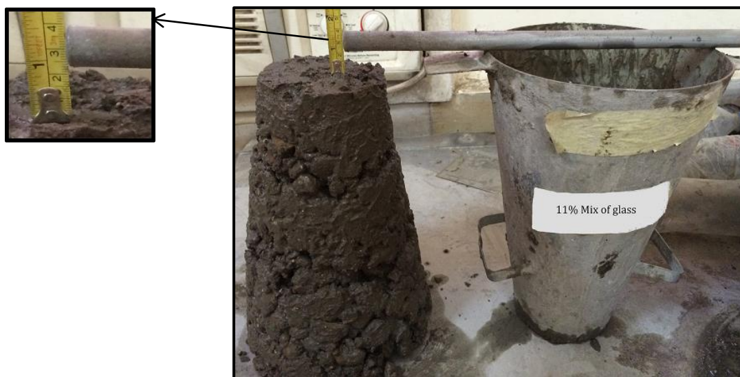
Figure -9: Slump measurement for 11% mix of glasses as a partial replacement of cement in the concrete mixture.
