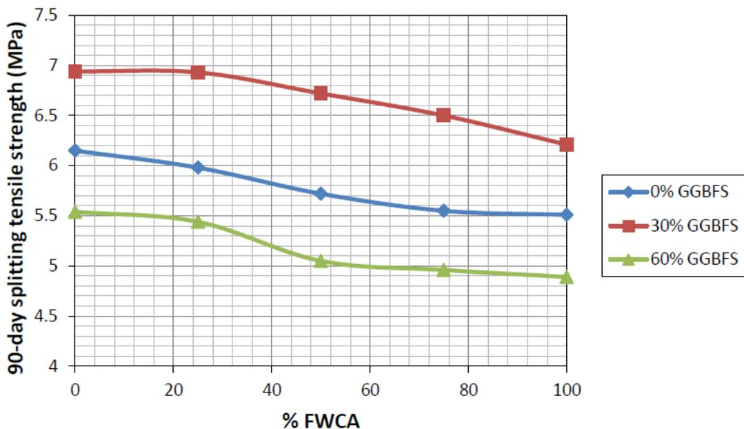
**Figure 8: Indirect tensile strength of the high strength mortars at 90 days.**
