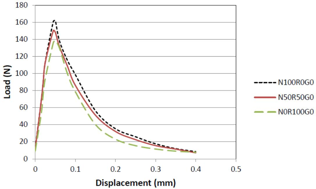
**Figure 10: Load-displacement plots for high strength mortars with 0% GGBFS at 28 days.**
