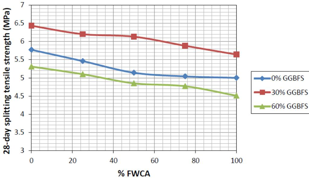
**Figure 7: Indirect tensile strength of the high strength mortars at 28 days.**
