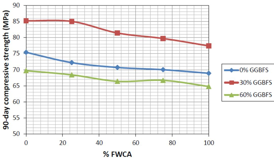
**Figure 5: Compressive strength of the high strength mortars at 90 days.**
