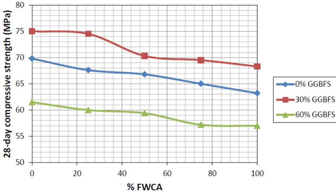
**Figure 4: Compressive strength of the high strength mortars at 28 days.**
