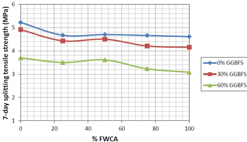
**Figure 6: Indirect tensile strength of the high strength mortars at 7 days.**
