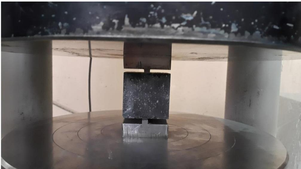
**Plate 1: Procedure for splitting tension test.**
