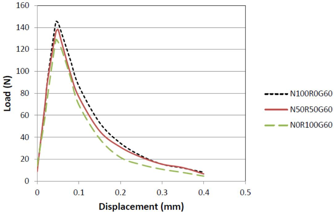
**Figure 12: Load-displacement curves for high strength mortars with 60% GGBFS at 28 days.**
