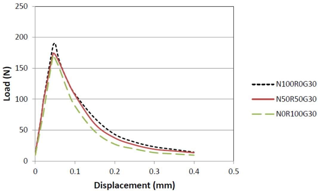
**Figure 11: Load-displacement curves for high strength mortars with 30% GGBFS at 28 days.**
