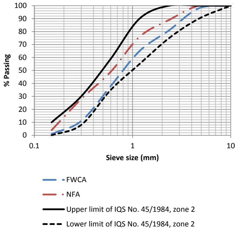
**Figure 1: Distribution of particle size of the fine aggregate.**
