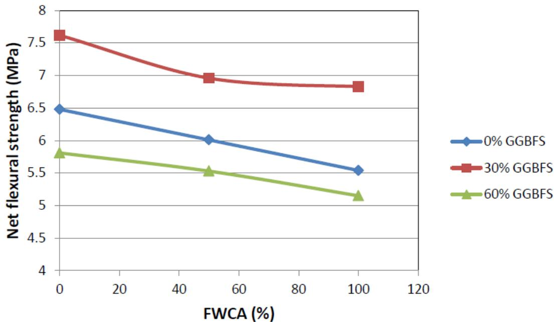
**Figure 9: Influence of FWCA percentage on the 28-day net flexural strength for different GGBFS levels.**
