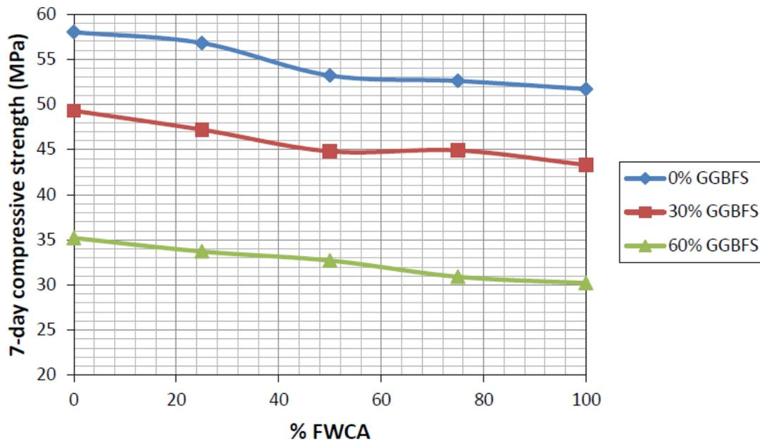
**Figure 3: Compressive strength of the high strength mortars at 7 days.**
