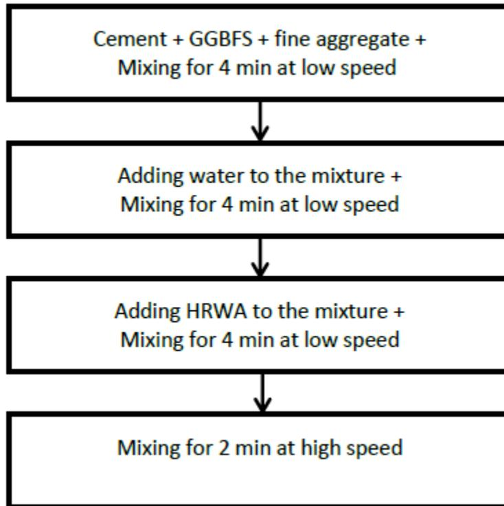
**Figure 2: Mixing procedure for mortars.**
