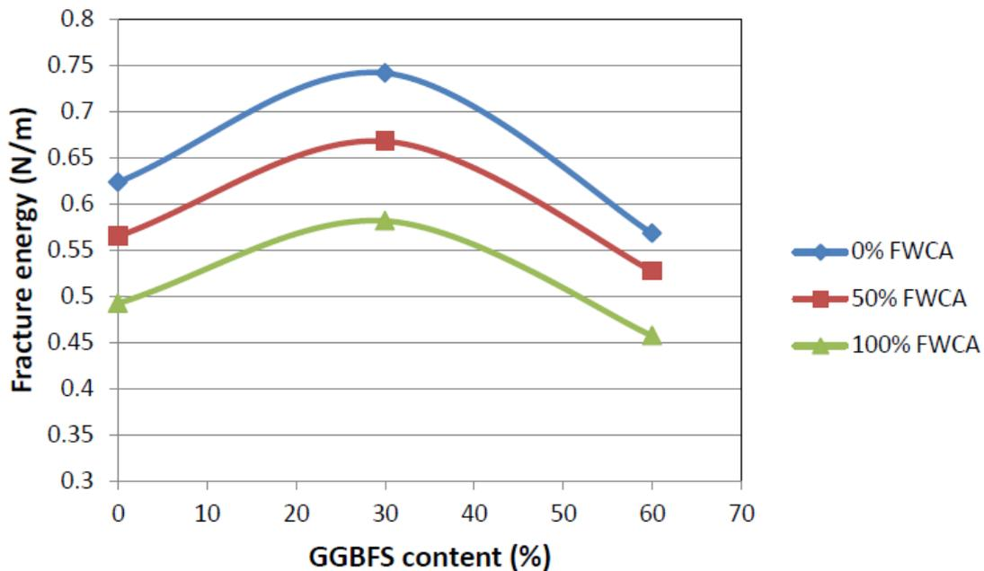
**Figure 13: 28-day fracture energy for different high strength mortars.**
