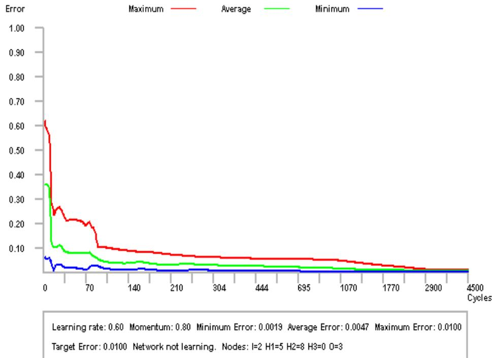
**Fig (3) Error Propagation for the 2,5,8,3 Architecture**
