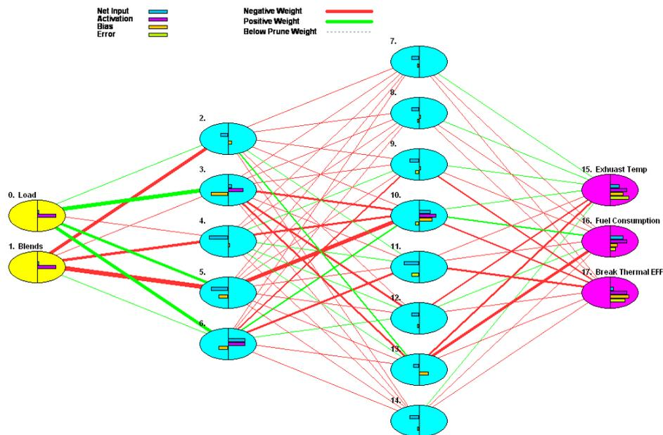
**Fig (2) The 2,5,8,3 Architecture Layers for Predicting Engine Performance**
