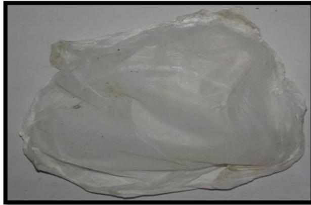
**Figure(1): air filter membrane after air filtration.**
