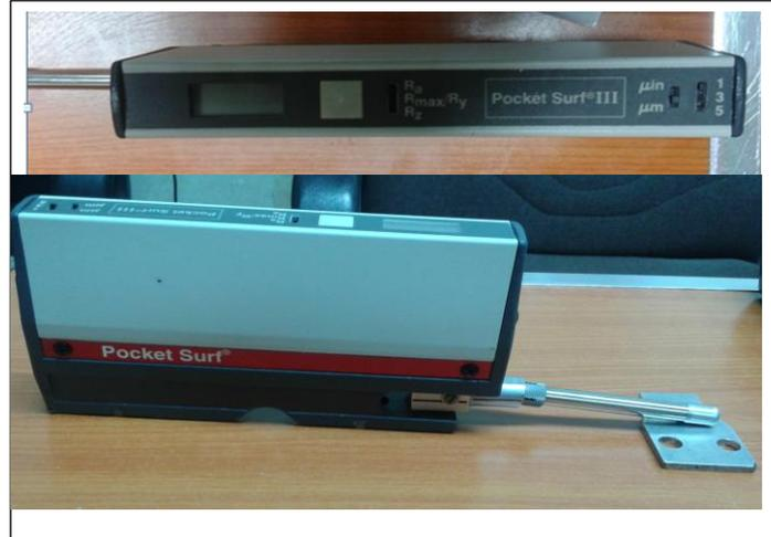
**Figure (5): Pocket surf IV Surface Roughness Testing Machine.**
