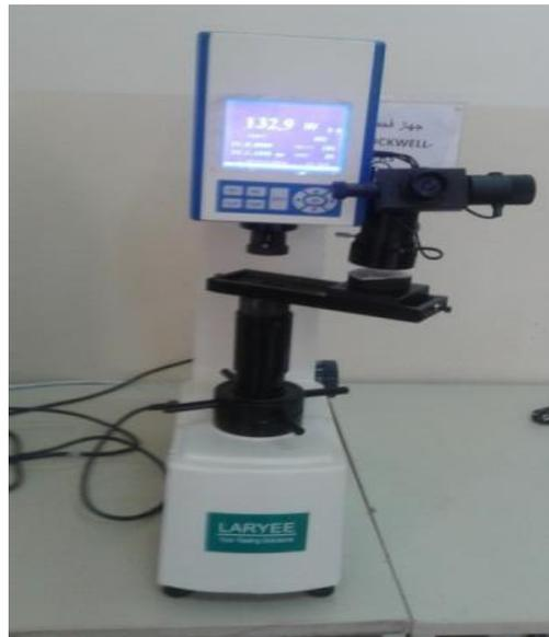
**Figure (4): Rockwell Hardness Testing Machine**
