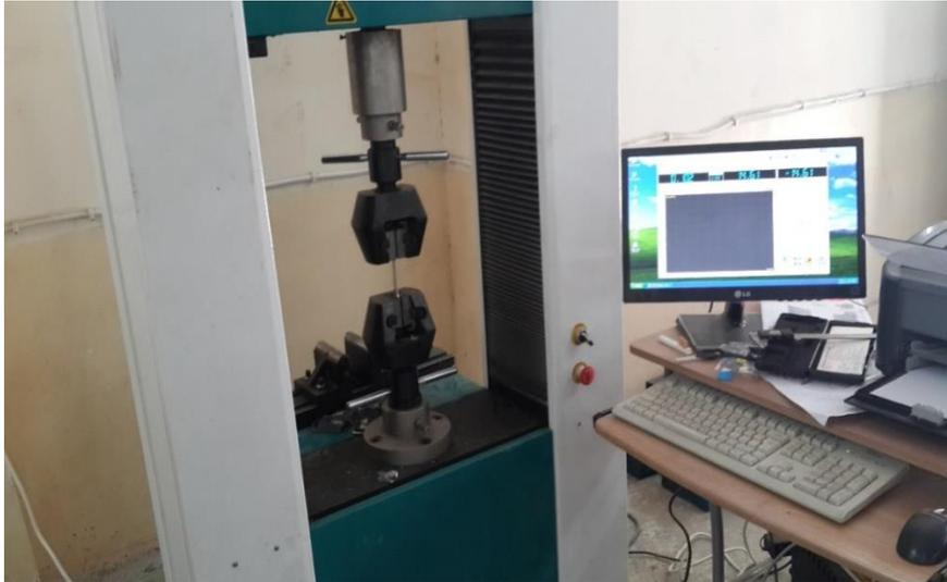
**Figure (3): Tensile Test Machine**
