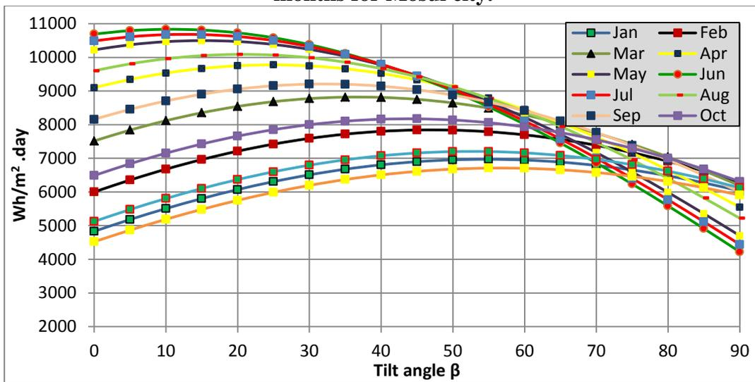
Fig. (3) Monthly total global solar radiation versus PV panel tilt angles over twelve months for Baghdad city.
