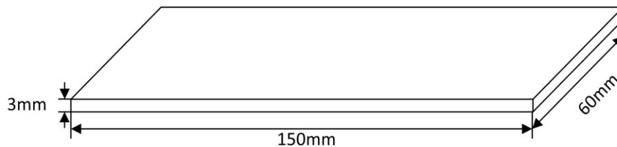
**Fig. 1 Geometry and dimensions of the composite plate**
