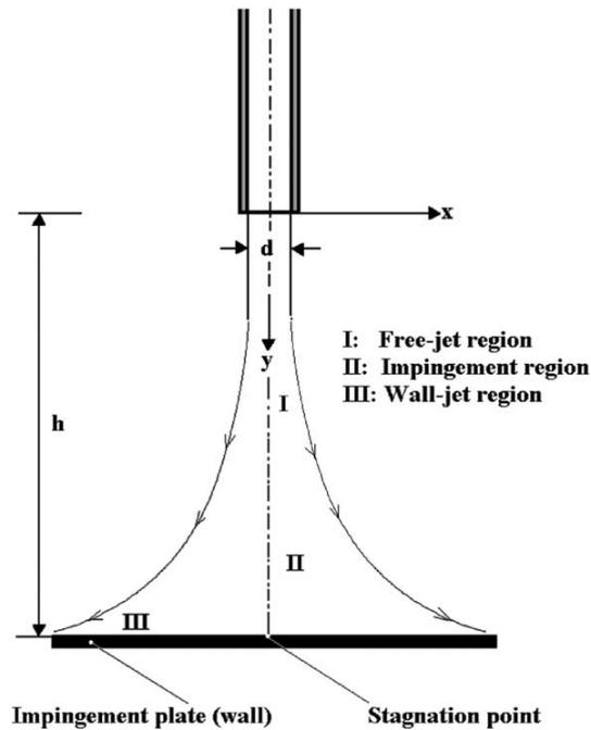
Fig. (1-7a) impinging jet configuration.
