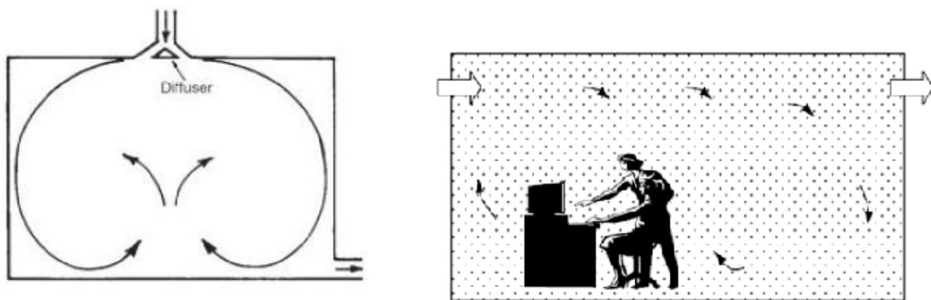
Fig. (1- 2) concept of mixing ventilation (Taghi Karimipناه. 2012)[13]
