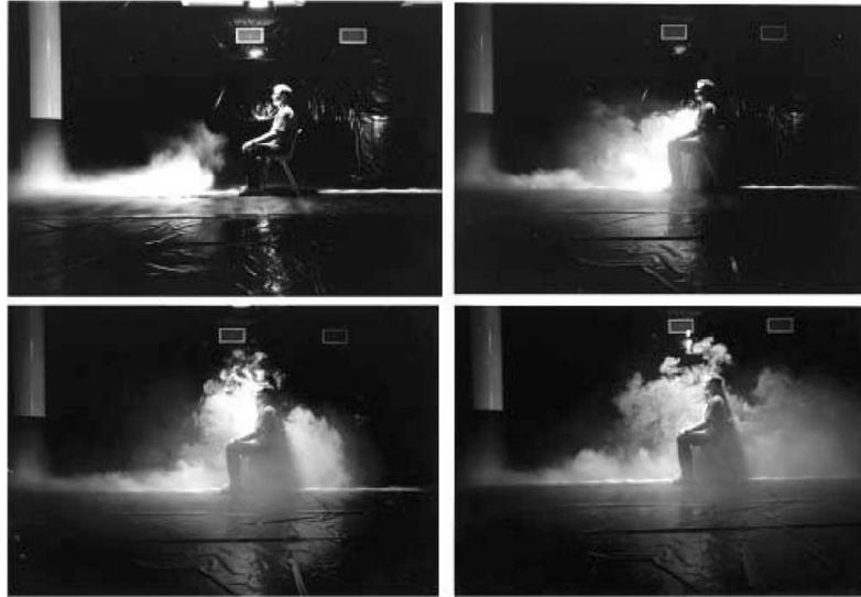
Fig. (1- 5) smoke visualization of impinging jet ventilation, (Taghi Karimipناه. 2012)[13]
