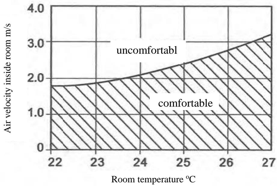
Fig. (1-8) thermal comfort zone (depend on air velocity), [36]
