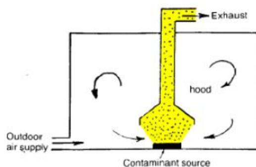
Fig. (1-1) concept of local exhaust ventilation system, [12]
