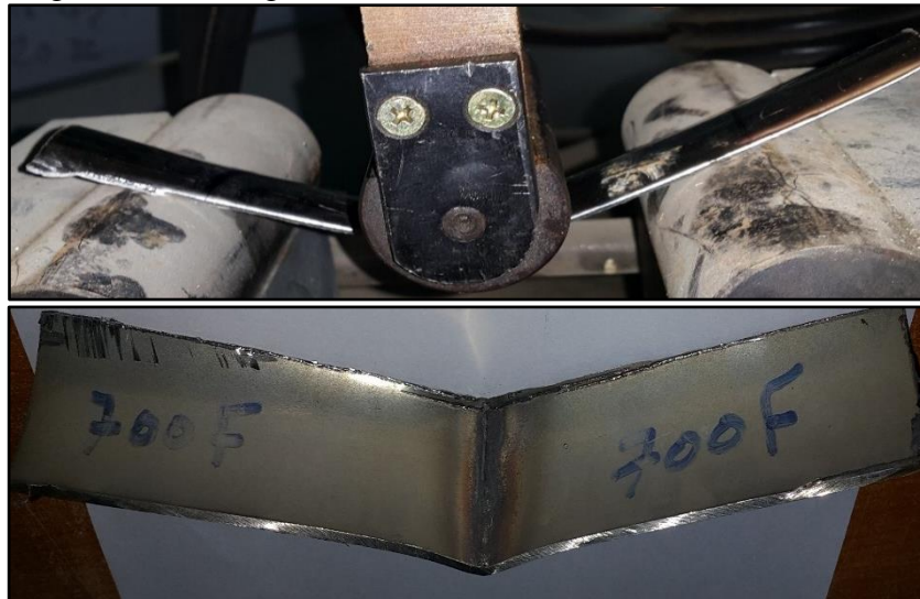
Fig. 9. Bending specimens through and after applying the load.
