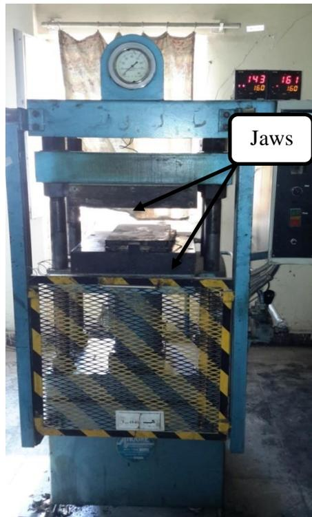
**Figure 3:** Thermal Hydraulic Press.
