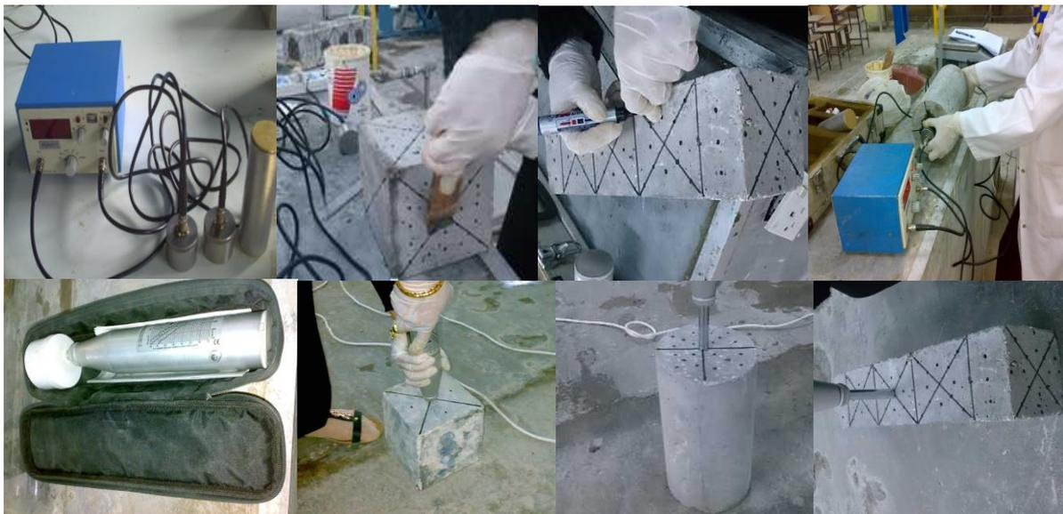
**Figure (4) Non-Destructive Tests Procedures of Specimens**
