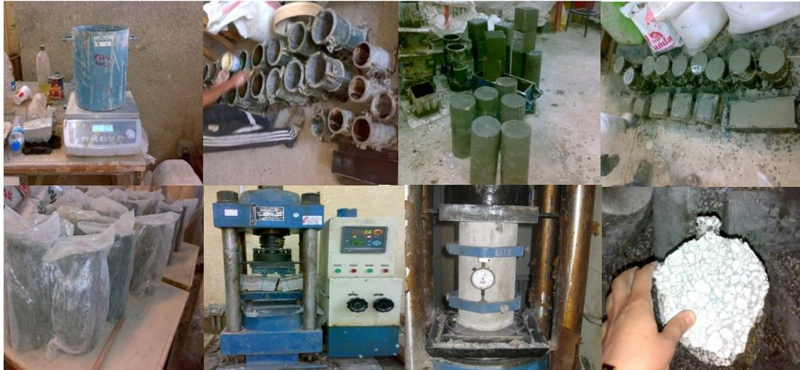
**Figure (3) Casting and Destructive Tests Procedures of Specimens**
