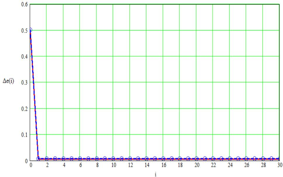
**Fig. 10. The dependence of the modulus of the error vector when the signal is extraction by the algorithm AbsoKurt (continuous blue) and AbsoKurtFP (continuous red with circles) from the iteration number for  $k = 0.9$ ; The kurtosis of the signal is 10; The kurtosis of the noise is equal to 1;  $\mu = 0.01$ ; The initial vector  $(0, 0)$ .**
