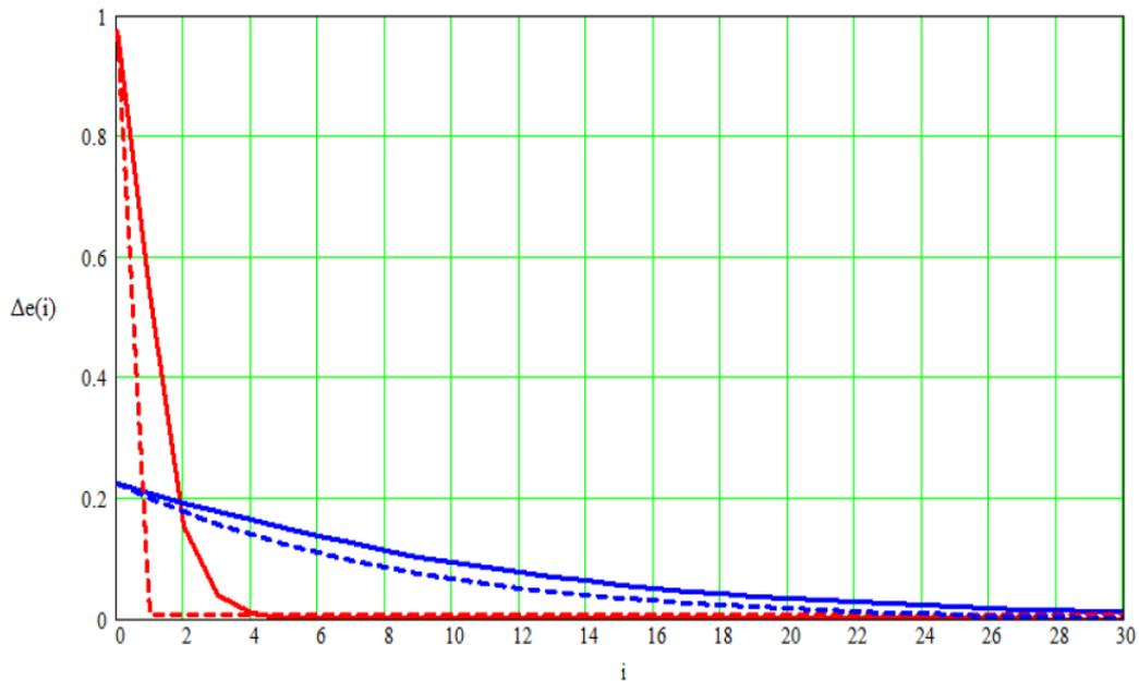
**Fig. 9. Dependence of the modulus of the error vector when the signal is extraction by the algorithm AbsoKurt (continuous blue - simulation, dotted –theoretical) And AbsoKurtFP (continuous red - simulation, dotted–theoretical) from the iteration number at  $k = 0.9$ ; The kurtosis of the signal is 10; The kurtosis of the noise is equal to 1;  $\mu = 0.01$ ; The initial vector (0, 1)**
