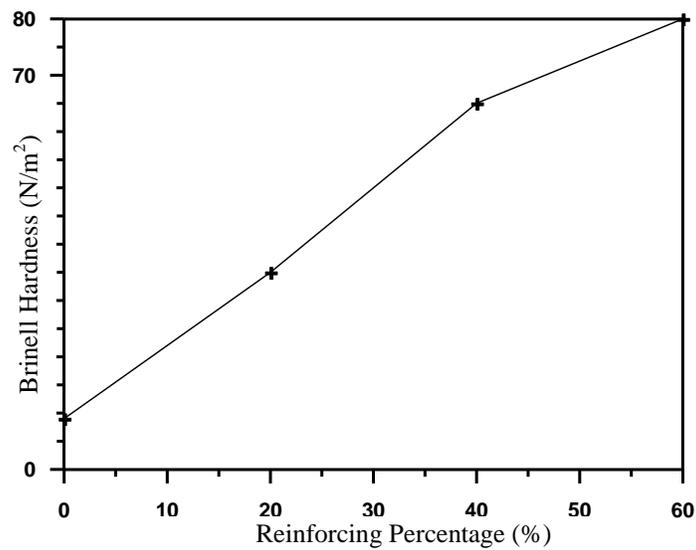
**Figure 4:** Hardness-reinforcing percentage curve of composite strength
