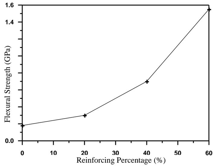
**Figure 3:** Flexural strength-reinforcing percentage curve of composite strength
