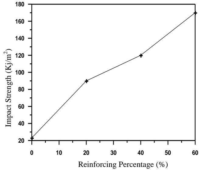
**Figure 1:** Impact strength-reinforcing percentage curve of composite strength
