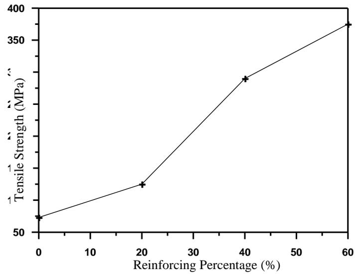
**Figure 2:** Tensile strength-reinforcing percentage curve of composite strength
