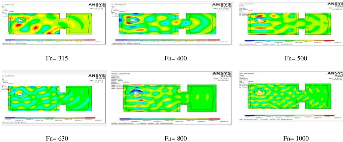
Figure (12): FEM Models Sound Pressure in Rooms at the One-Third Octave Frequency.
