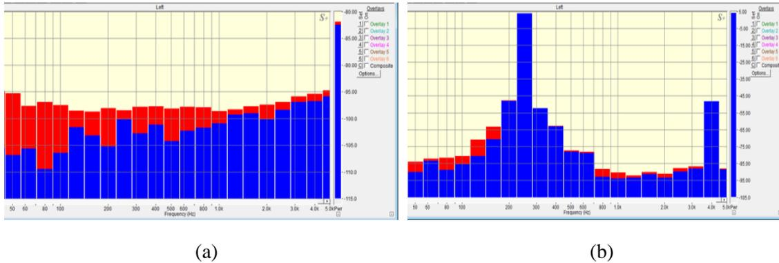
**Figure (16) ): Experimental (SPL) for Two Rooms When Close the Partition Between Rooms by Two Sandwich Panel ,(a) Resaved Room.(b) Sources Room.**
