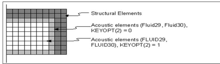
**Figure (4): 2-D Acoustic Model [11].**
