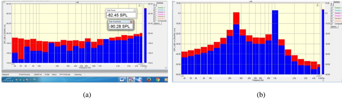
**Figure (19): Experimental (SPL) for Two Rooms When close the Partition Between Rooms by One Sandwich Panel 100mm Thickness for Core, (a) Resaved Room. (b) Sources Room.**
