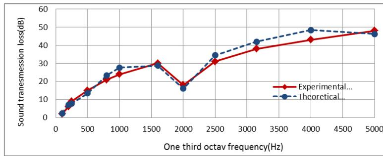
**Figure (17) Comparison Theoretical and Experimental (STL), Closed the Partition Between Two Rooms by Using Two Sandwich Panel (50) mm for Thickness for One Third Octave.**
