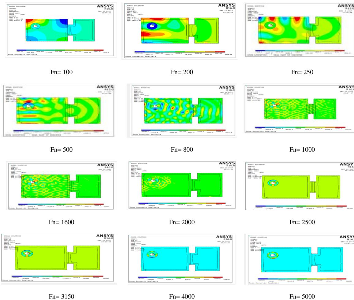
**Figure (21):FEM Models Sound Pressure for Case Study Closed the Partition Between Two Rooms by Using One Sandwich Panel (100) mm Thickness Core.**
