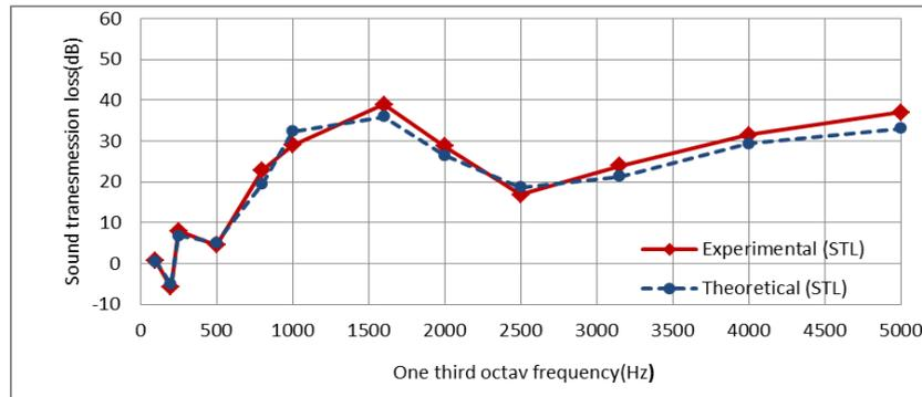
**Figure (14): Comparison Theoretical and Experimental STL Results Between Two Rooms for One Third Octave.**
