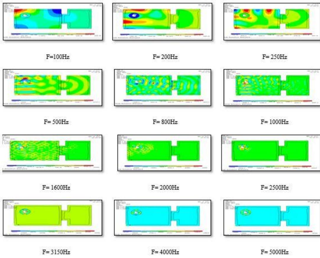
**Figure (15): FEM Models (Meshes and Sound Pressure) for Case Study One Sandwich Panel (50) mm for Thickness a Core. Between Two Rooms for One Third Octave.**
