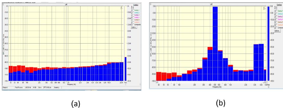
Figure (13): Experimental (SPL) for Two Rooms When close the Partition Between Rooms by One Sandwich Panel 50mm Thickness for Core,(a) Resaved Room.(b) Sources Room.
