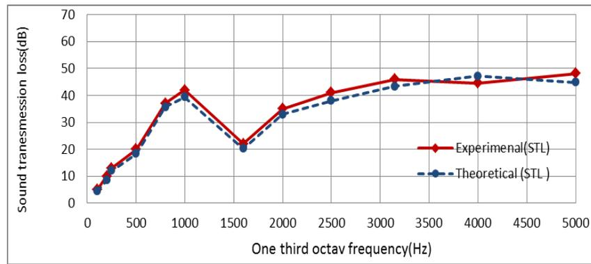
**Figure (20): Comparison Theoretical and Experimental, STL Closed the Partition by One Sandwich Panel.**
