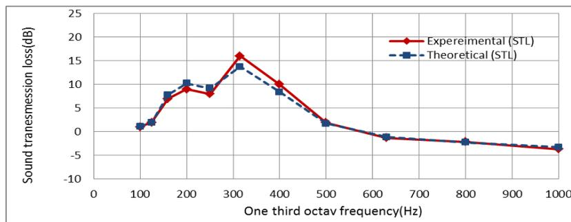
**Figure (11): Comparison Theoretical and Experimental STL Results For Open the Partition Between Two Rooms.**
