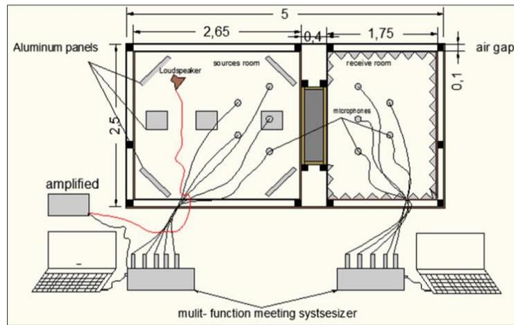
**Figure (6): Design of Test Room for Transmission Loss (all Dimensions m).**
