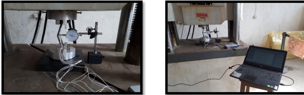
Fig. 14: Calibration between measuring deflection by dial gauge with strain gauge.
