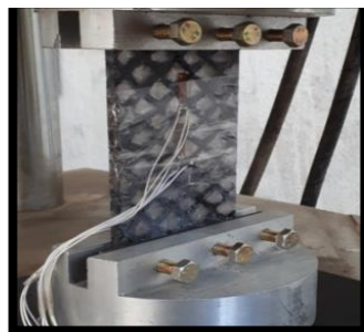
Fig. 13: Buckling load and deflection for CFRP composite laminated plates measuring by using strain gauges.
