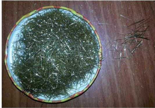
**Plate (1): Ultra Fine Steel Fiber MSF Used in This Investigation**
