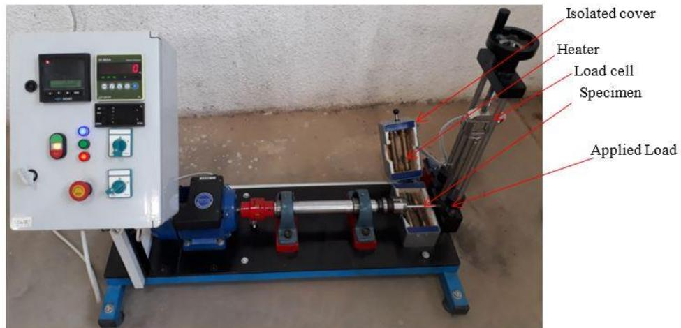
Figure (2): Fatigue testing machine.
