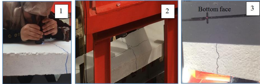
Plate 4. Crack Patterns of Composite castellated beam 25%
