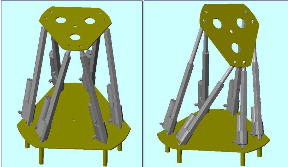
**Fig (15): Platform at initial and final position.**
