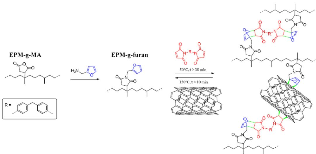
**Fig. 2 Furan functionalization and bismaleimide (BM) cross-linking of EPM-g-furan and the integration of CNT fillers via covalent interactions in the thermoreversibly cross-linked network of the nanocomposite [15].**
