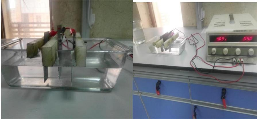
**Figure 2 shows the electrodeposition Process of zinc.**
