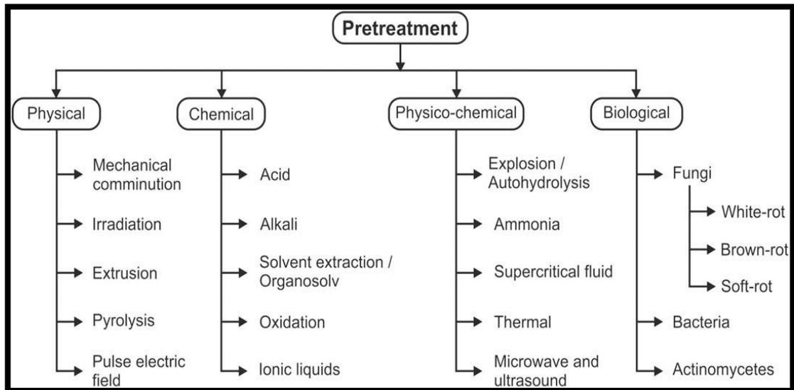
**Figure 3. Scheme for various pretreatment of biomass[30].**
