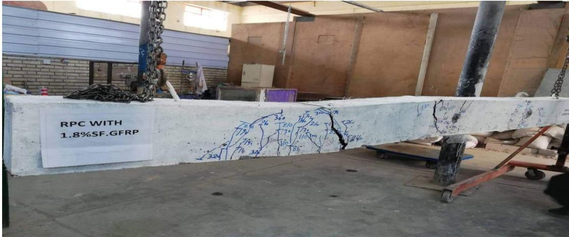
**Fig. 14. Crack Patterns of RPC (1.8%V.F with GFEP Bar)**
