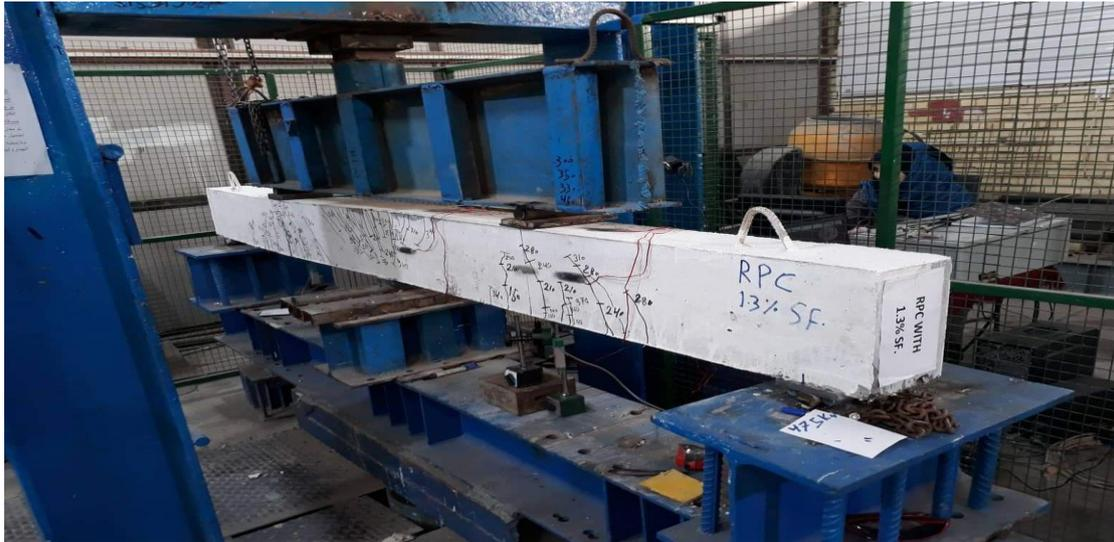
**Fig. 11. Crack Patterns of RPC (1.3%V.F)**
