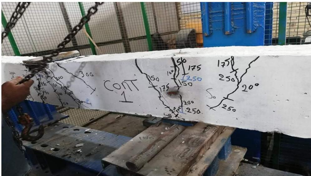
**Fig. 7. Crack Patterns of Beam B1 (NC)**
