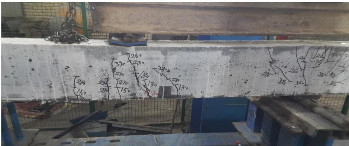
**Fig. 13. Crack Patterns of RPC (2.5%V.F)**
