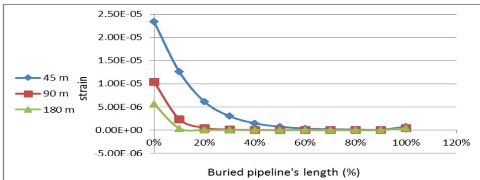
**Fig. ( 8 ) Strains–percentage of buried pipeline's length relationship for different values of length.**
