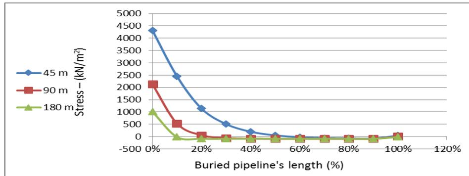
**Fig. ( 7 ) Stresses–percentage of buried pipeline's length relationship for different values of length.**
