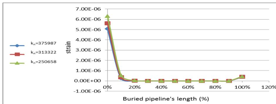
**Fig. ( 11 ) Strain–percentage of buried pipeline's length relationship for different values of ( $k_n$  and  $k_s$ ).**
