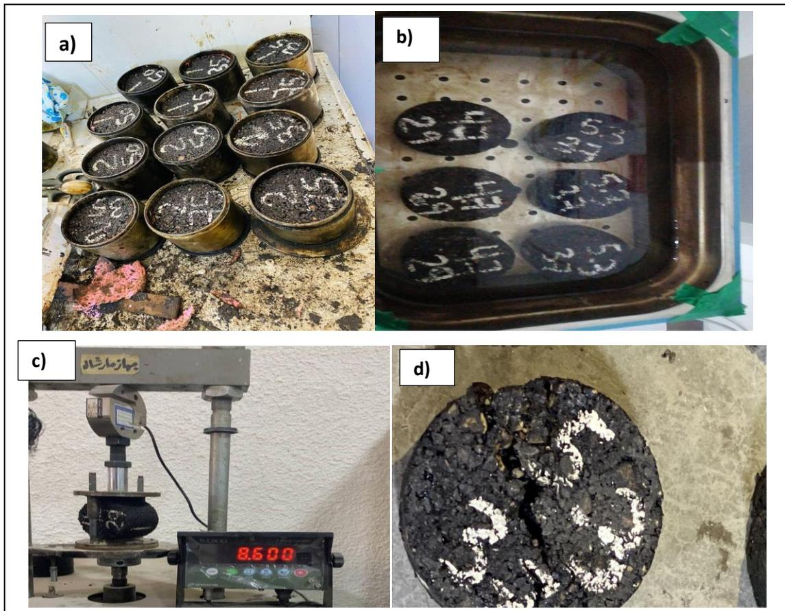
**Plate 2. Steps for indirect tensile testing a) Preparing tested samples b) Treated in a water bath c) Examining the model with a tensile tester d) sample after failure.**
