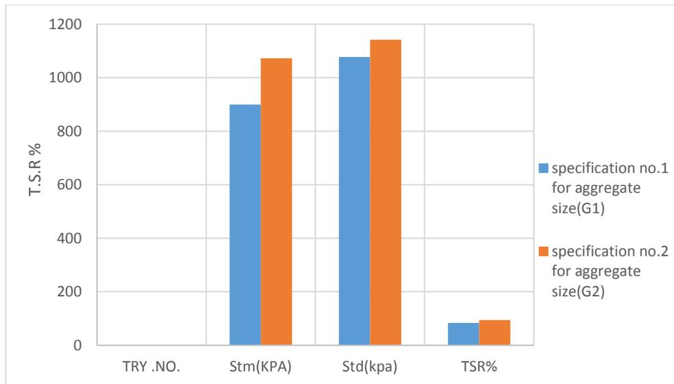
. Figure 3. A comparison of the results of the TSR test for G1 and G2
