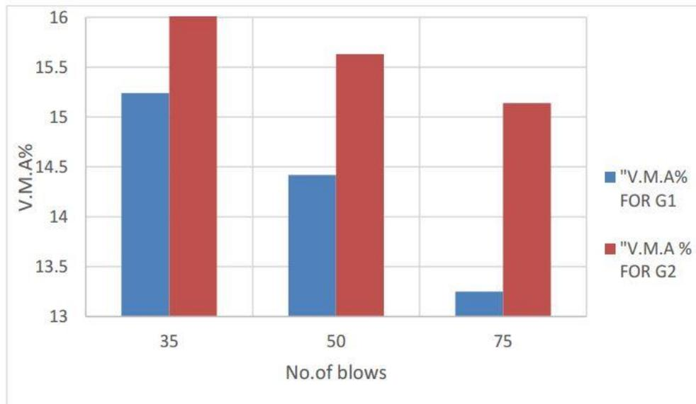
**Figure 6. Test results of V.M.A %.**
