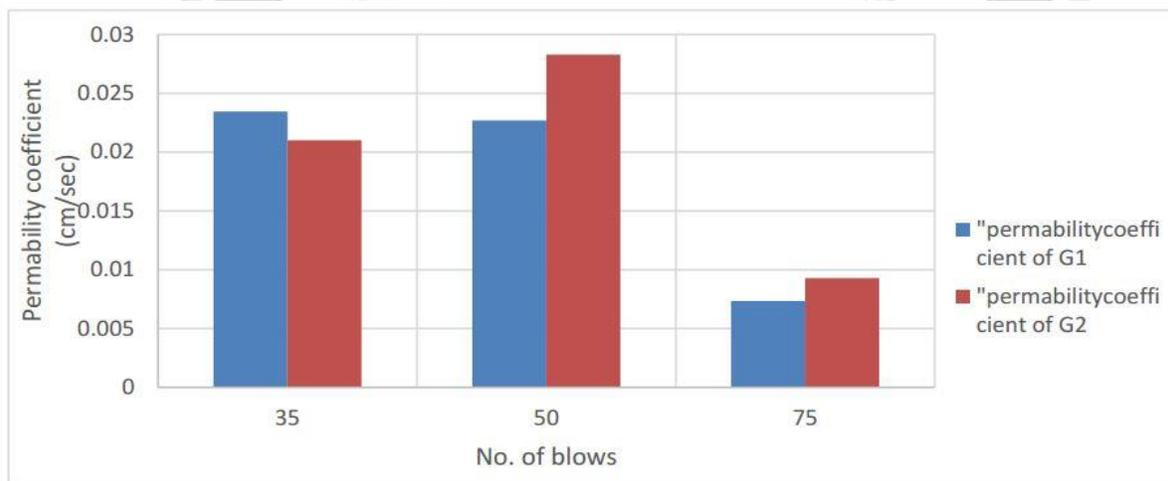
Figure 8. A comparison of the results of the permeability coefficient test for the  $G_1$  and  $G_2$ .
