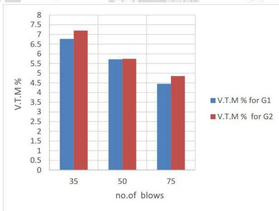
Figure 5. Test results of V.T.M %
