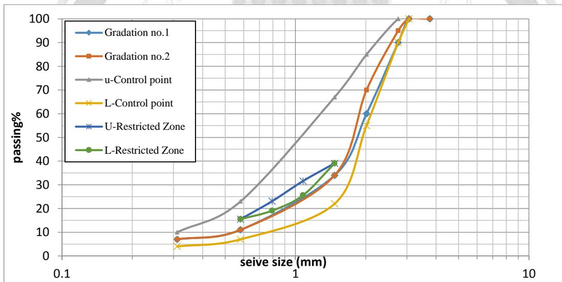
**Figure 1. Trail Gradations for Surface Layer.**
