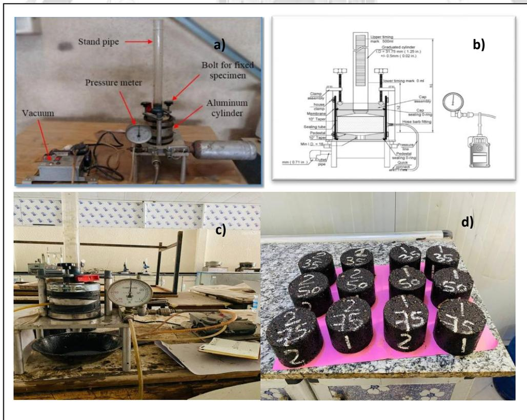
**Plate 1. The schematic Diagram and setup of HMA permeability test a) The schematic Diagram of HMA permeability test (Florida Department of Transportation) b) Permeability apparatus c) Mixing Samples d) The method of checking the device.**
