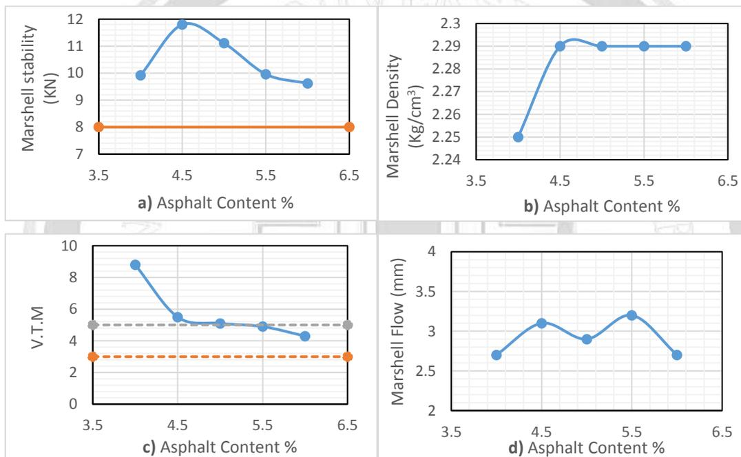
**Figure 2. Determination of OAC according to Marshall method for G<sub>1</sub>: a) Relationship between Stability and AC%; b) Relationship between Unit weight and AC%; c) Relationship between Air void and AC%; d) Relationship between Flow and AC%.**
