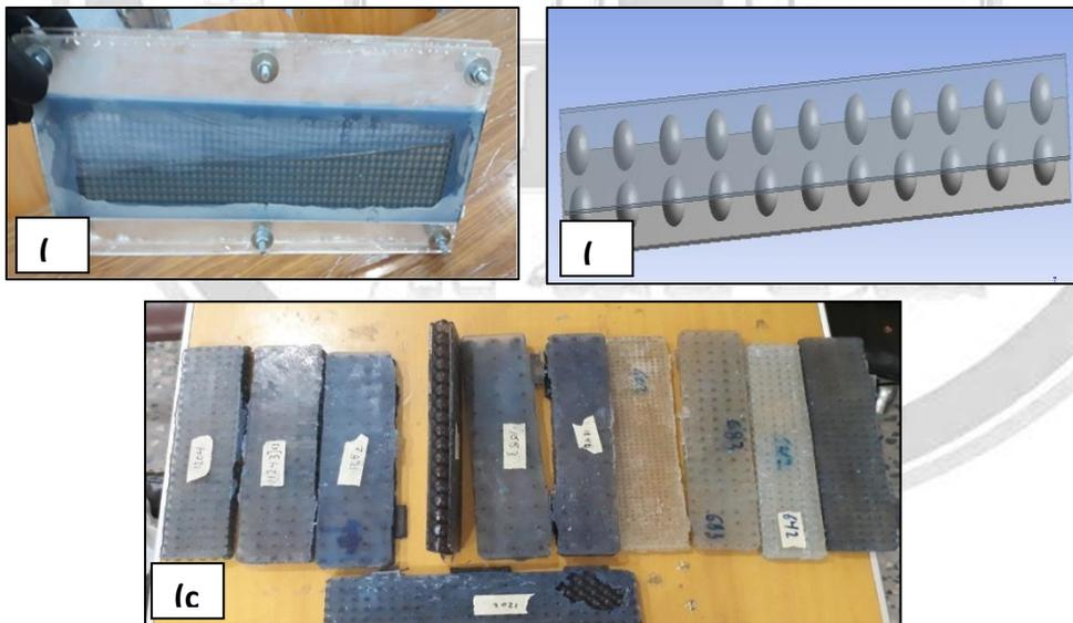
**Figure 1 : (a) mold of wax with spheres cavities, (b) sandwich sphere structure, (c) fifteen samples of sandwich sphere structure.**
