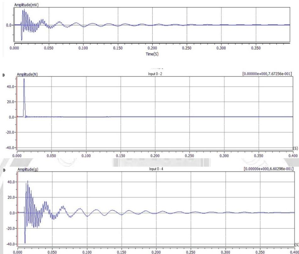
**Figure 4: The excitation force and structure response in the time domain.**
