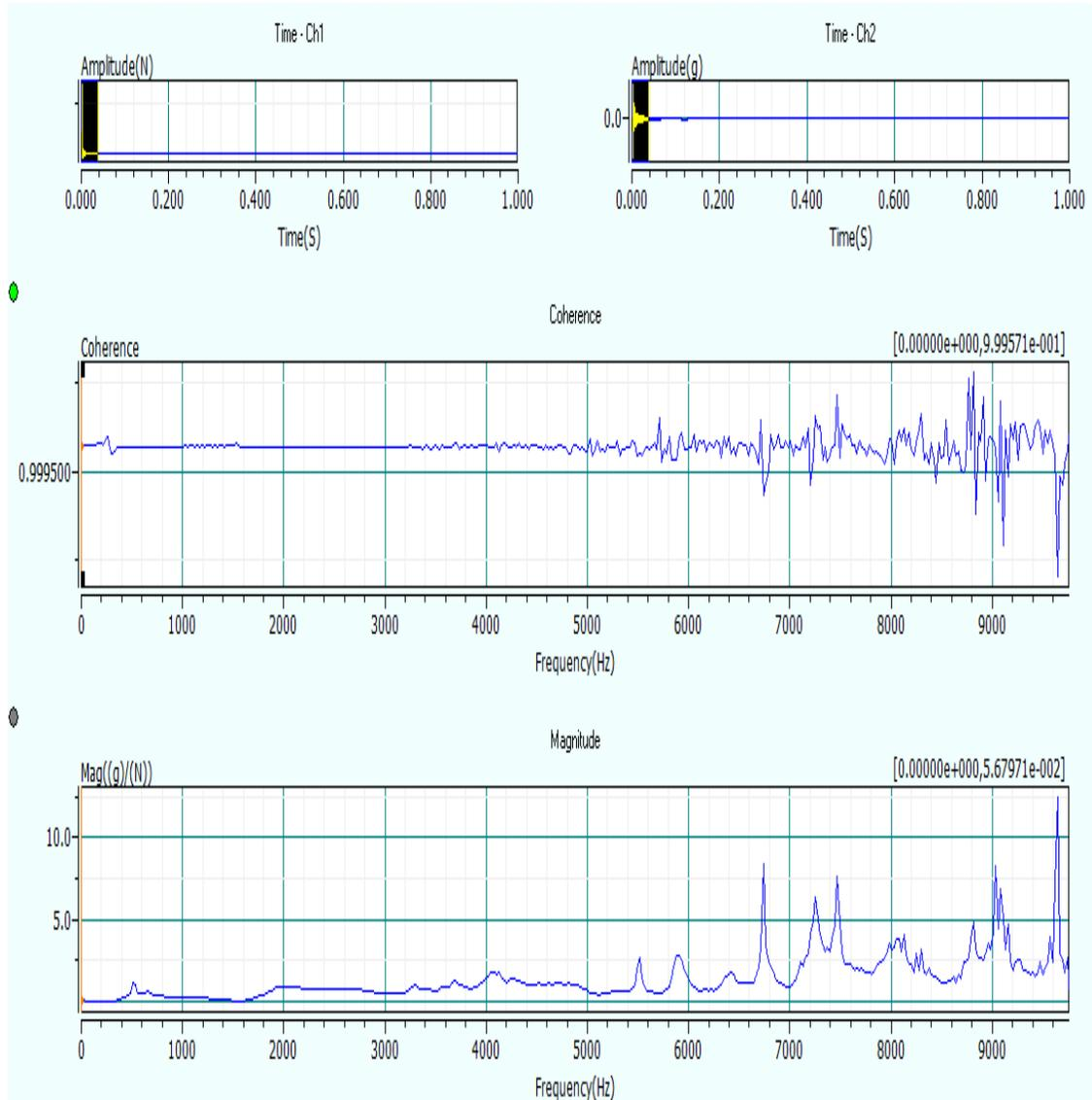
**Figure 5: The FRF and coherence diagram.**
