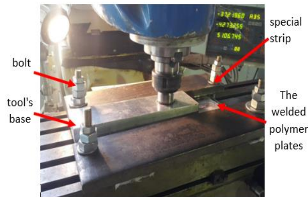
Figure 1: Special attachments fixed on the machine milling
