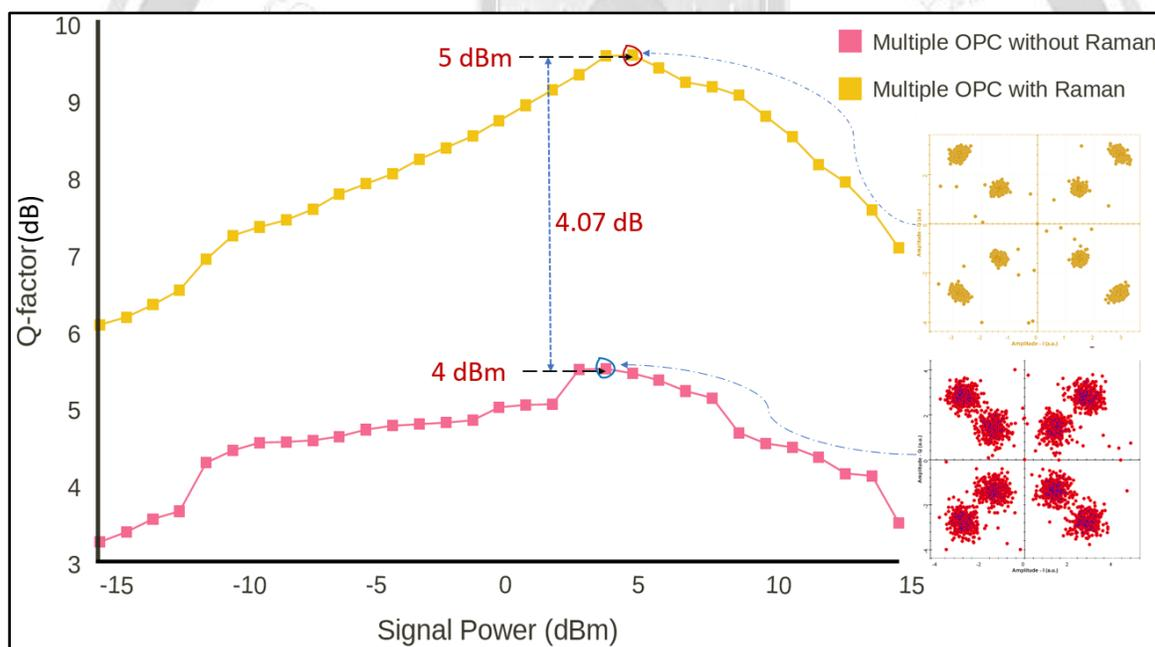
**Fig. 12. Signal power vs. Q-factor and eye diagram for the middle channel (ch.8) of multiple OPC module with and without Raman amplifier**
