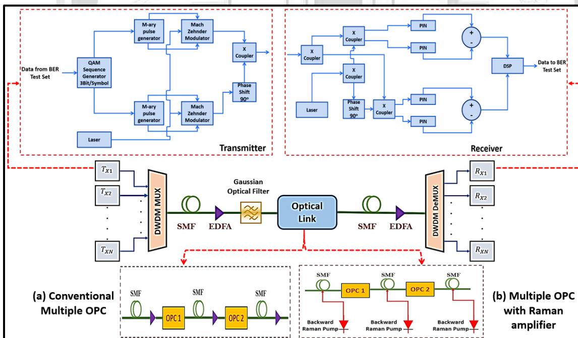
Fig. 6. 8QAM system model of multiple OPC with and without Raman amplifier
