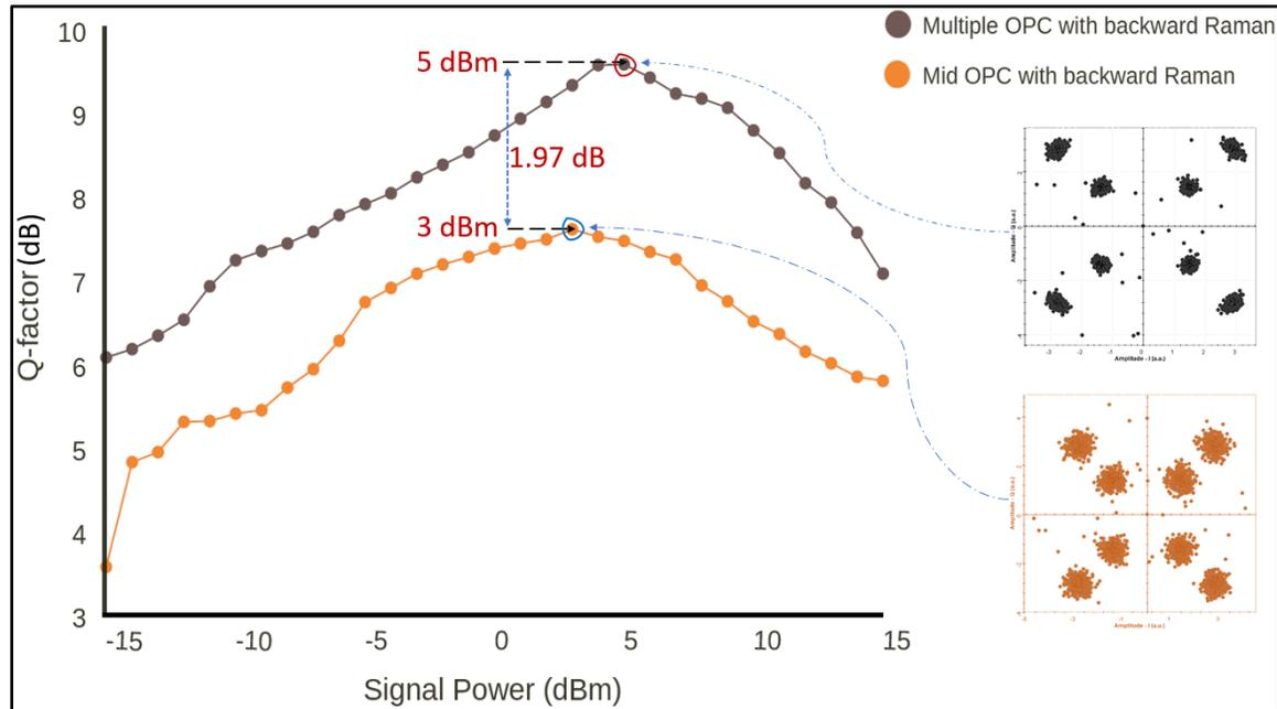
**Fig. 13. Signal power vs. Q-factor and eye diagram for the middle channel of mid and multiple OPC module with Raman amplifier**
