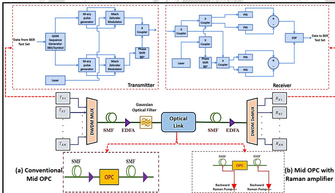
**Fig. 5. model of an 8QAM mid OPC system with and without a backward Raman amplifier with transmitter part (upper left) and receiver part (upper right)**
