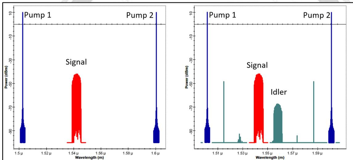
**Fig. 9. The spectrum of the 8-QAM signal with OPC (left) before pass through HNLF (right) after pass HNLF**
