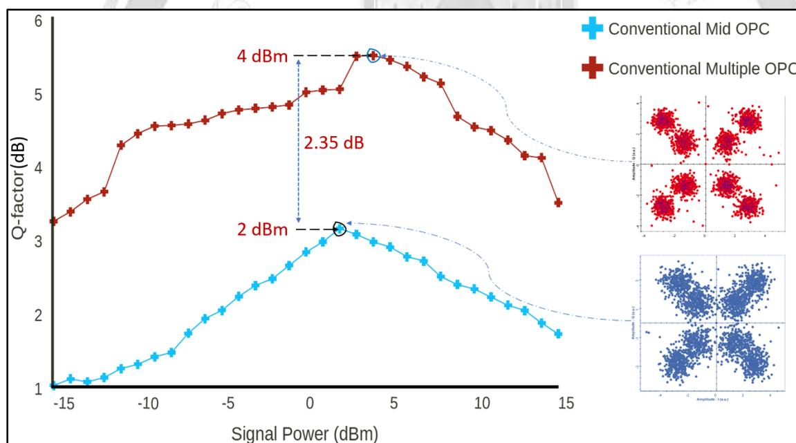
**Fig. 11. Signal power vs. Q-factor and eye diagram for the middle channel of conventional mid and multiple OPC module**
