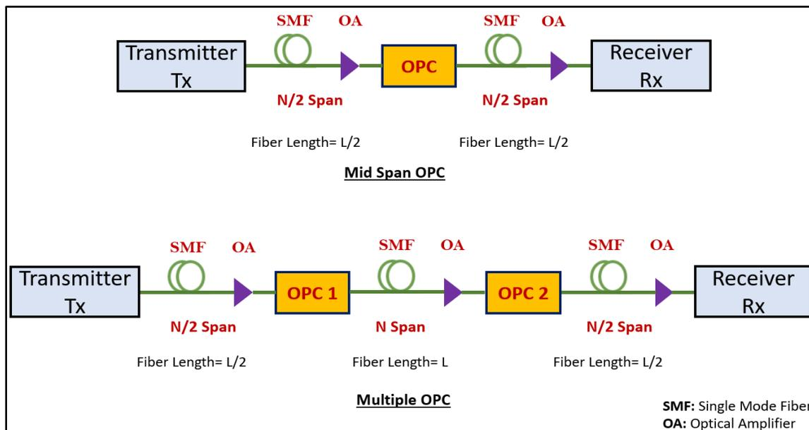
Fig. 3. OPC implementation: mid span schemes (upper) and multiple span schemes (lower)
