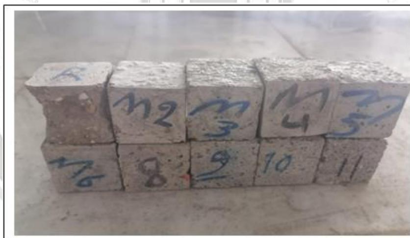
Figure 8. Plate represent the mode of failure of cubes sample under compression test
