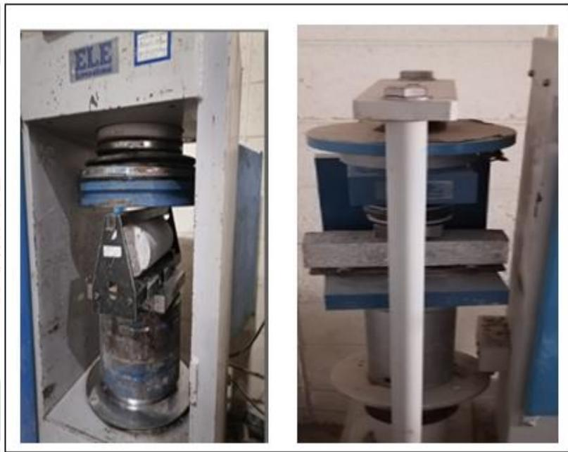
Figure 2. Splitting and flexural tests machine
