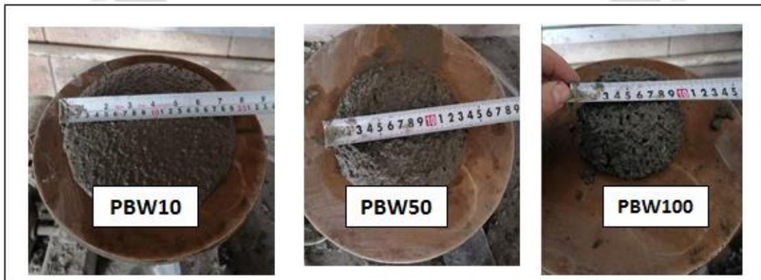
Figure 4. Samples from slump flow examination
