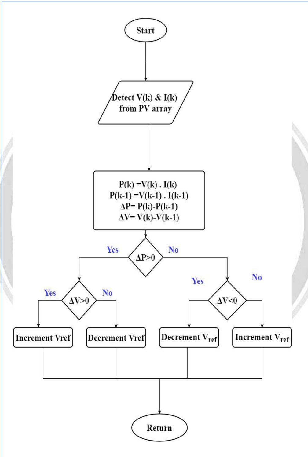
Figure 9. P&amp;O Algorithm
