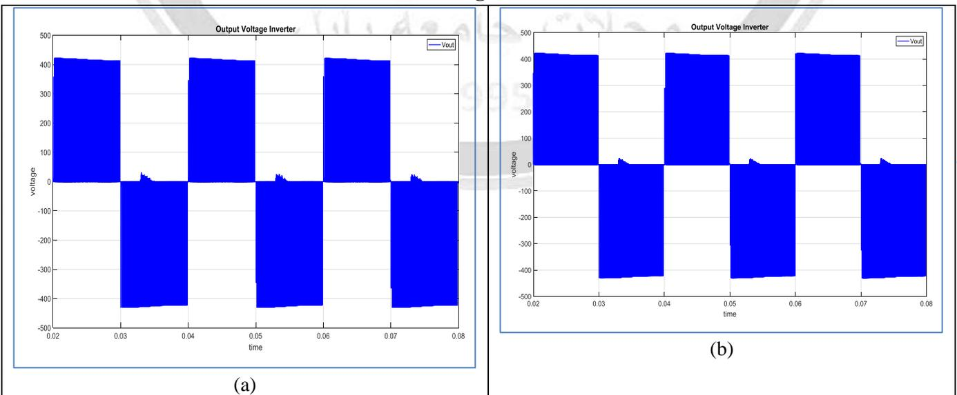
**Figure 15.  $V_{out}$  of 3 level ISI-NPC inverter under (a) P&O algorithm and (b) ANN algorithm**
