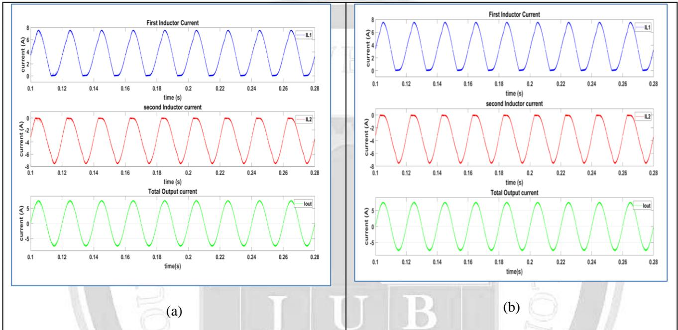
**Figure 14.  $I_{L1}$ ,  $I_{L2}$  and  $I_{out}$  of 3 level ISI-NPC inverter under (a) P&O algorithm and (b) ANN algorithm**
