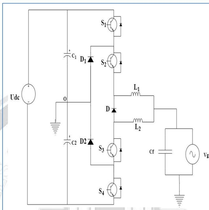
**Figure 3. Three-level Improved SI-NPC [28]**
