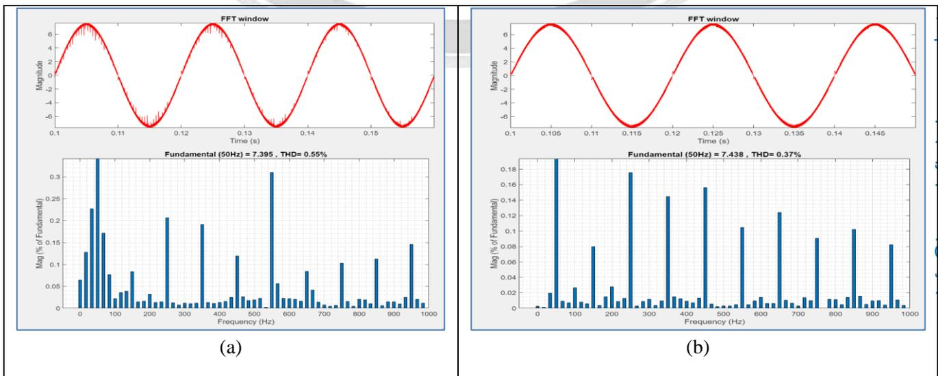
Figure 21. FFT analysis of current THD under (a) P&O algorithm and (b) ANN algorithm
