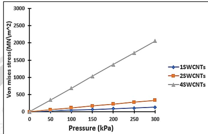
Figure 4. Pressure vs Von Mises Stress at Single-walled CNT
