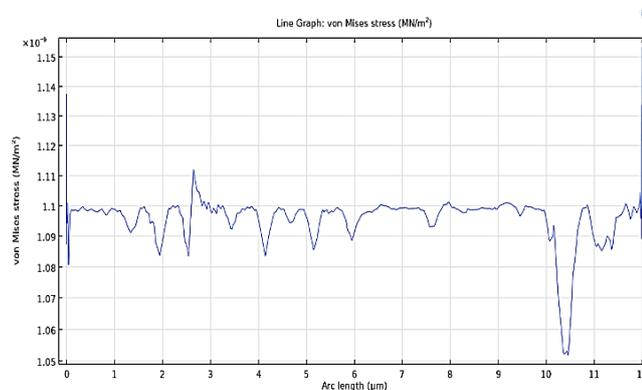
Figure 7. Arc Length vs Von Mises Stress of SWCNTs
