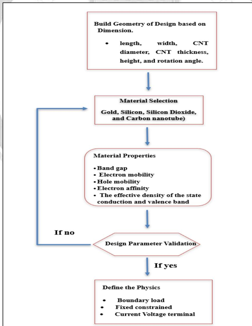
Figure 2. Flowchart of Simulation Work of SWCNTs based Pressure Sensor in COMSOL Multiphysics.
