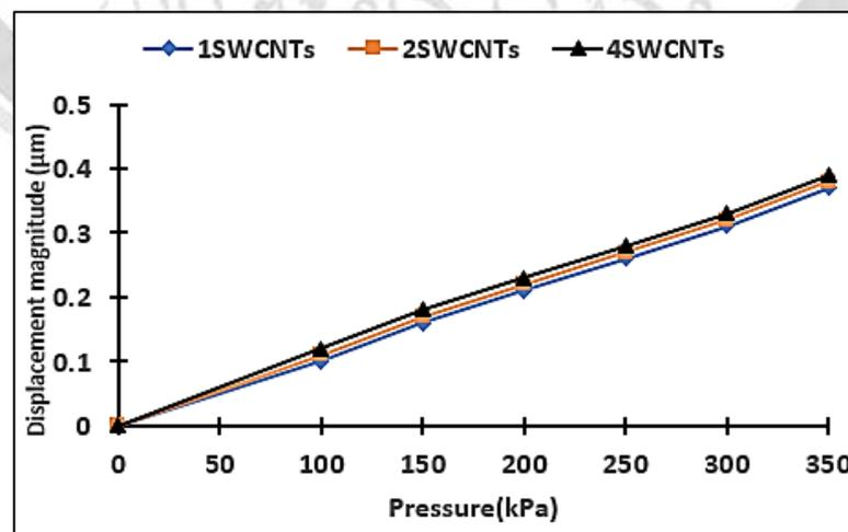
Figure 5. Pressure vs Displacement of Single-walled CNT
