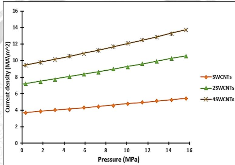
Figure 6. Relationship between Pressure and Current Density of SWCNTs
