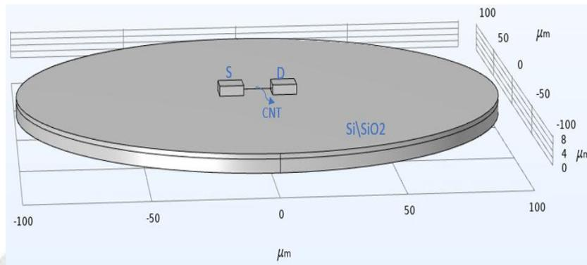
Figure 1. Geometry of SWCNT pressure sensor
