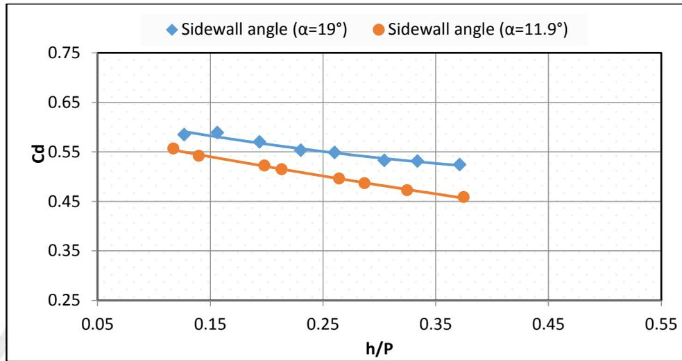
**Fig. (8): Relation of the Cd and h/P for two models of combined labyrinth weirs-gate (P=15cm).**
