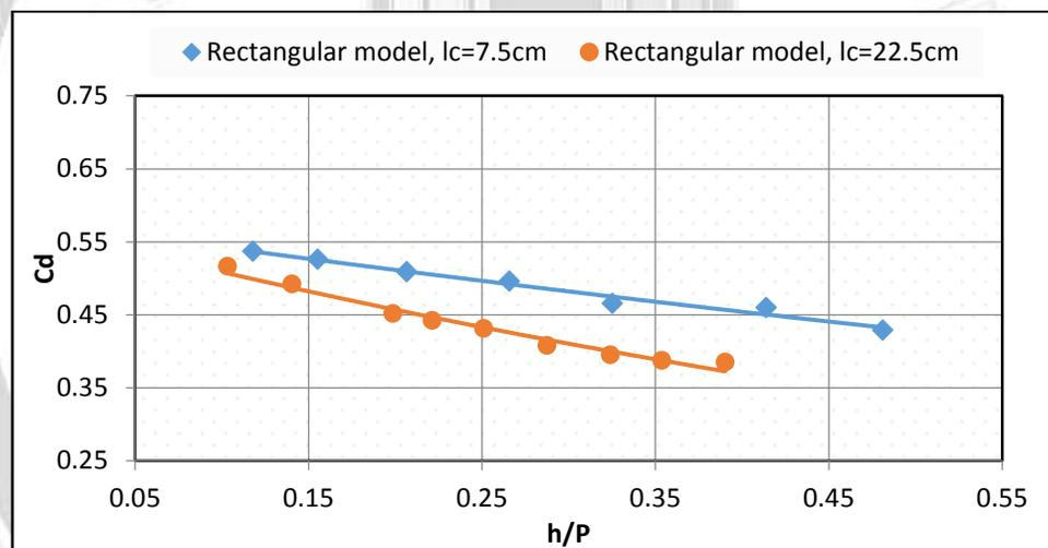
**Fig.(5): Relation of the value of Cd and h/P for the two models combined labyrinth weirs-gate.**
