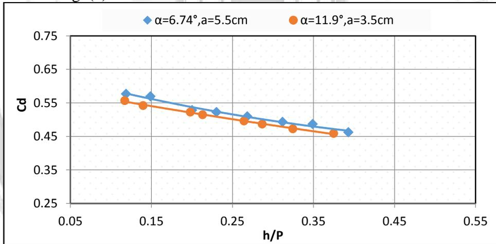
**Fig. (7): Relation of the Cd and h/P for combined labyrinth weirs-gate (P=15cm).**
