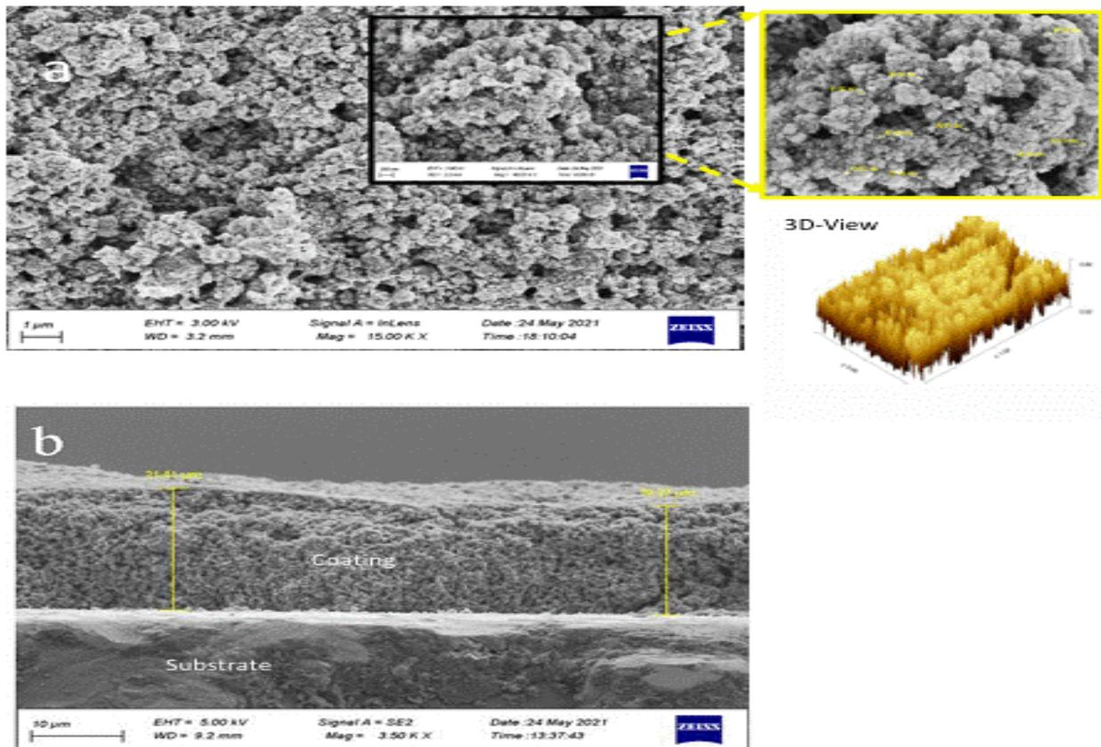
**Fig.5 FE-SEM micrograph (a) and (b) cross sectional views of TiO<sub>2</sub>-CS deposited at 300 sec at 50% DC.**
