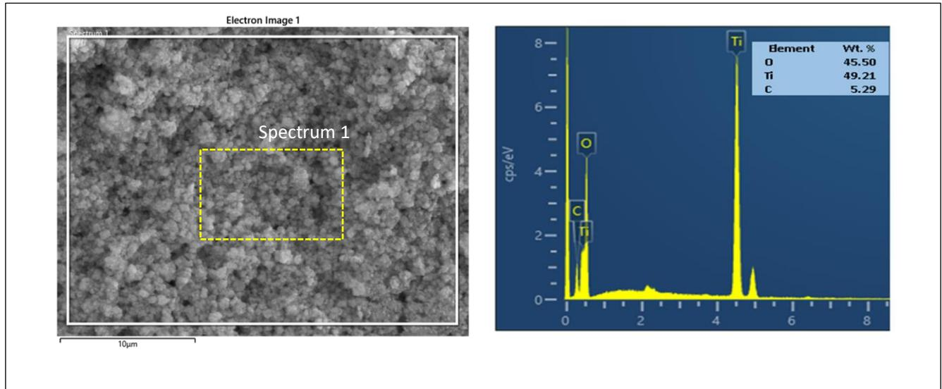
**Fig.6. The EDX spectra of the TiO<sub>2</sub>-CS composite coating.**
