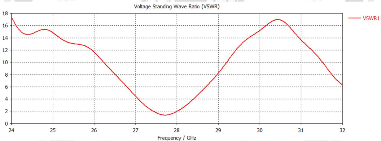
Figure 9: The VSWR of the 1x2 hexagon patch antenna array
