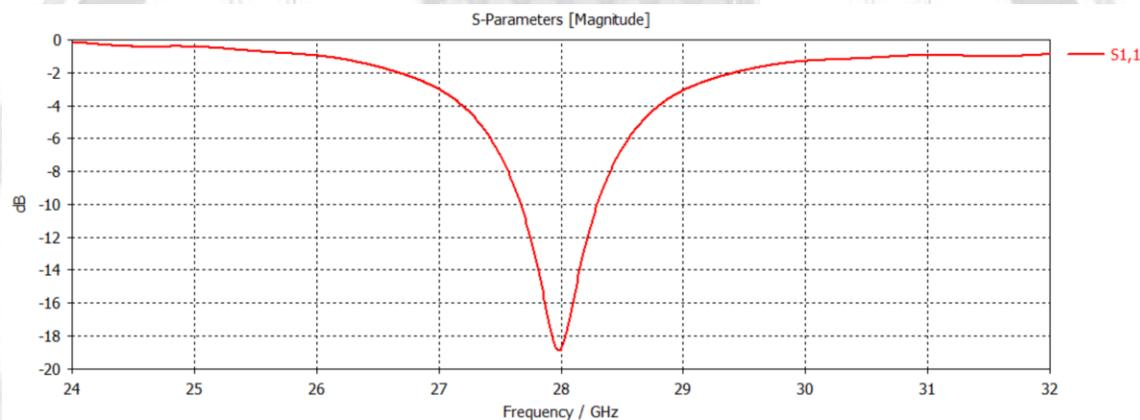
**Figure 4: The reflection coefficient of the hexagon patch antenna**
