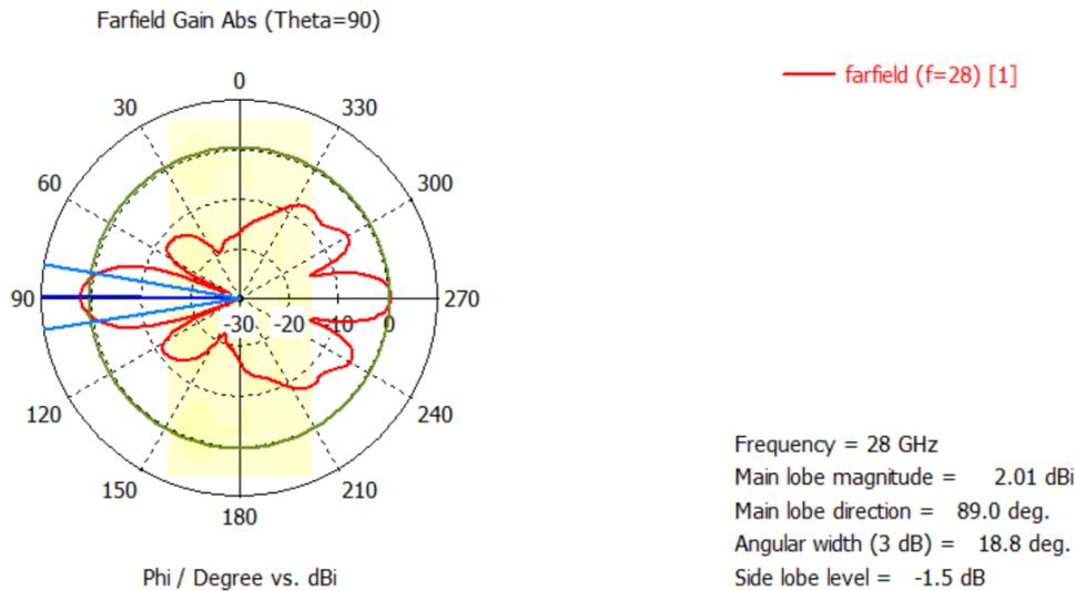
**Figure 15: 1-D farfield of the 1x4 hexagon patch antenna array**
