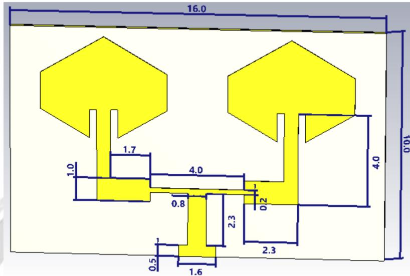
Figure 2: The designed 1x2 hexagon patch antenna array
