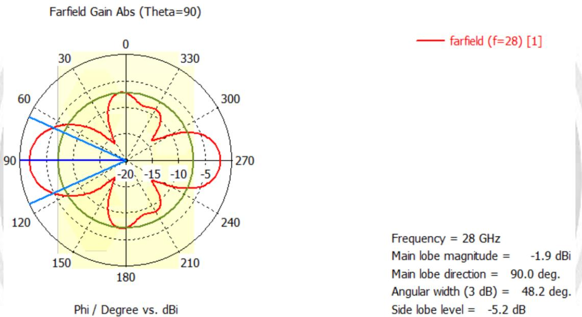
Figure 11: 1-D farfield of the 1x2 hexagon patch antenna array
