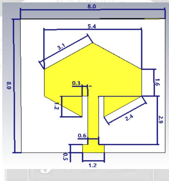
**Figure 1: The designed hexagon patch antenna**
