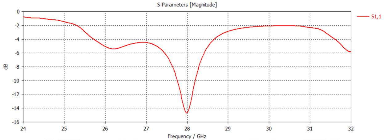
Figure 12: The reflection coefficient of the designed 1x4 hexagon patch antenna array
