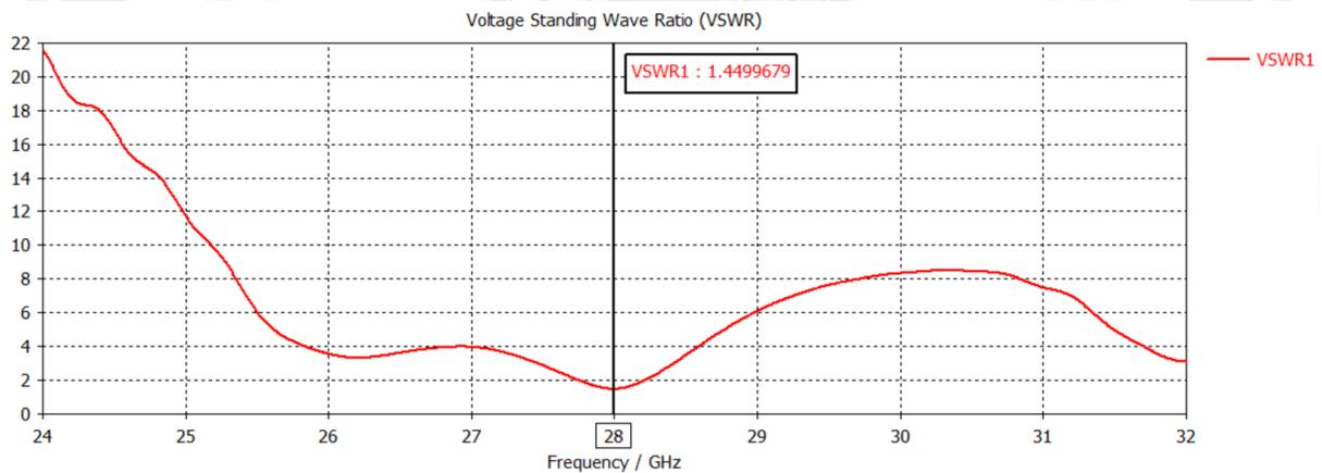
Figure 13: The VSWR of the 1x4 hexagon patch antenna array
