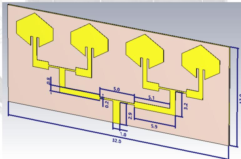
Figure 3: The designed 1x4 hexagon patch antenna array
