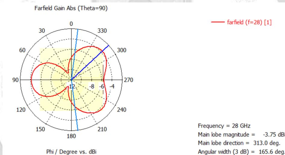
**Figure 7: 1-D farfield of the hexagon patch antenna**
