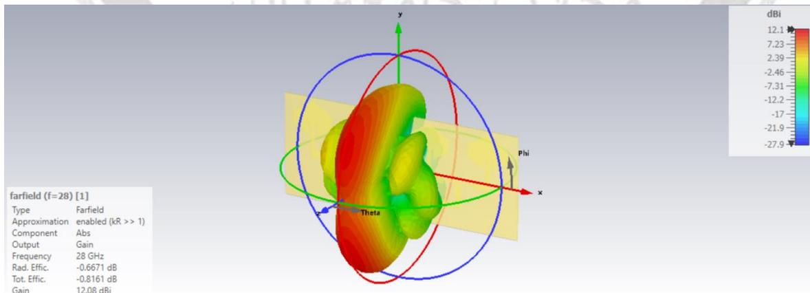
Figure 14: 3-D farfield of the 1x4 hexagon patch antenna array
