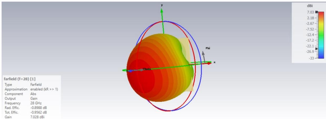
**Figure 6: The 3-D farfield of the hexagon patch antenna**
