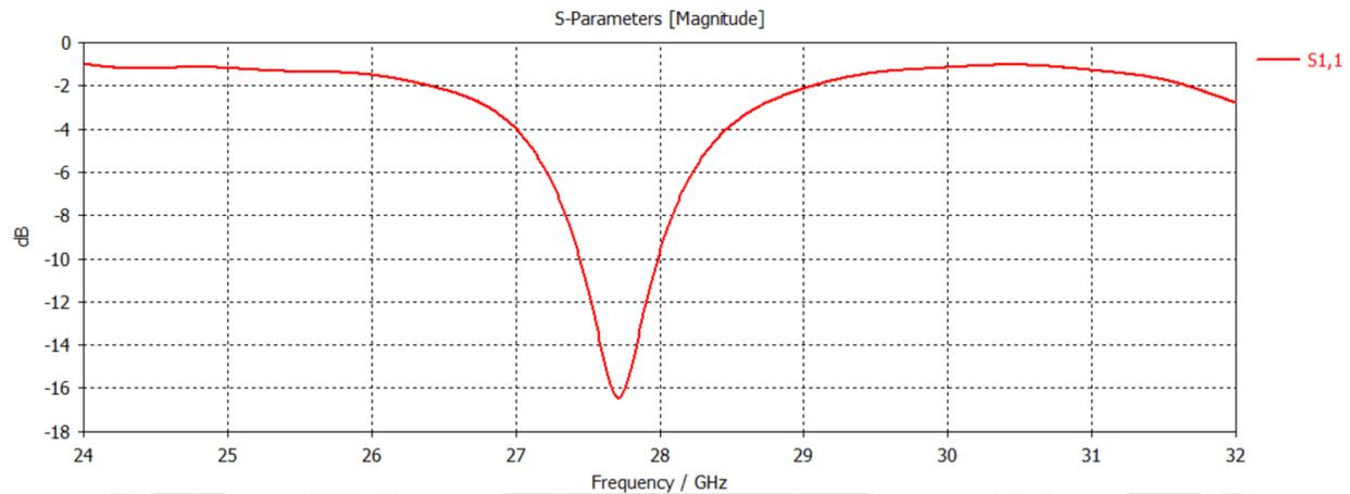
Figure 8: The reflection coefficient of the 1x2 hexagon patch antenna array
