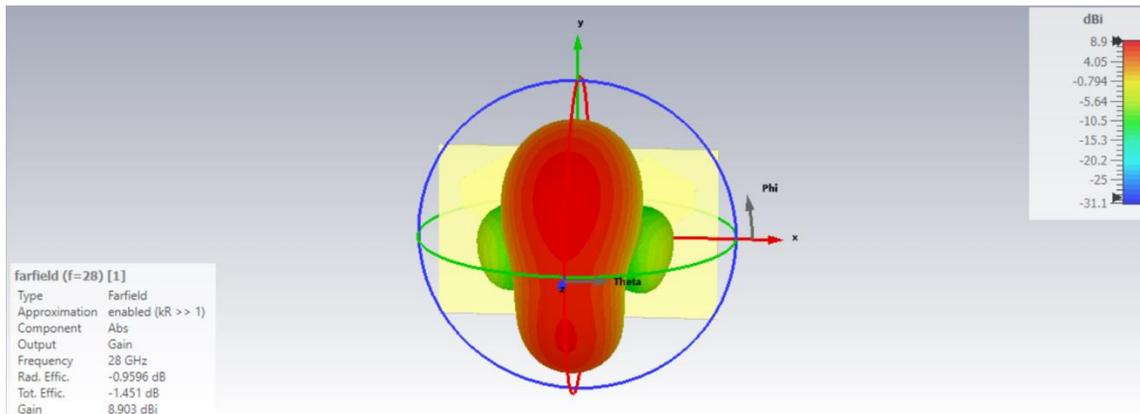
Figure 10: 2-D farfield of the 1x2 hexagon patch antenna array
