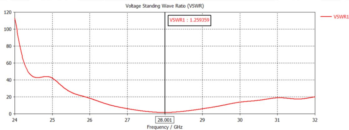
**Figure 5: The VSWR of the hexagon patch antenna**
