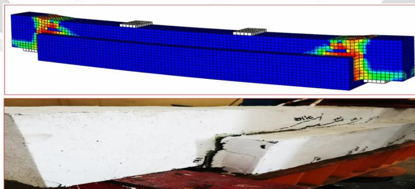
Fig. 17 b: Crack pattern of RU.
