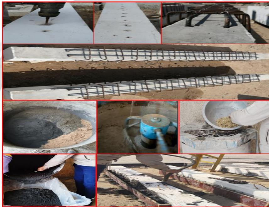
**Fig. 2: Steps of reinforced beam for UHPC and mixing procedure.**
