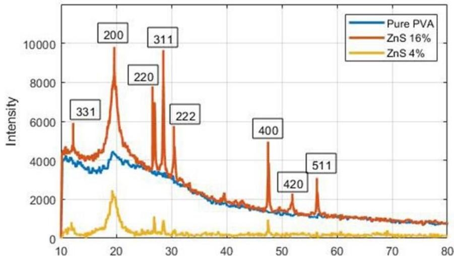
Figure 1 : XRD PVA with 4 and 16wt% ZnS NPs.
