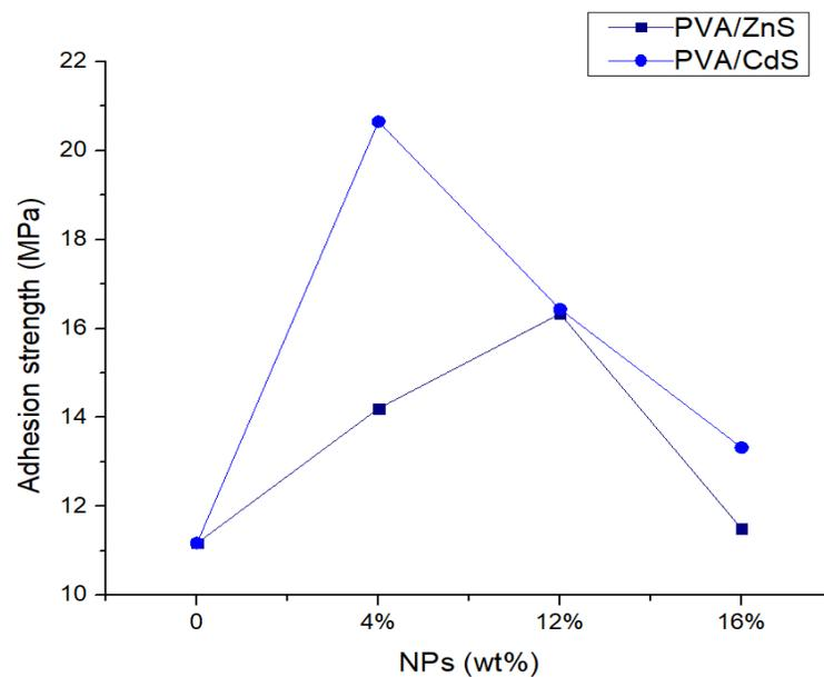
Figure 4 :Adhesion strength values for PVA/NPs (with different ratio).
