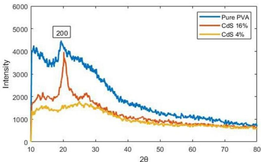
Figure 2 : XRD PVA with 4 and 16wt% CdS NPs.
