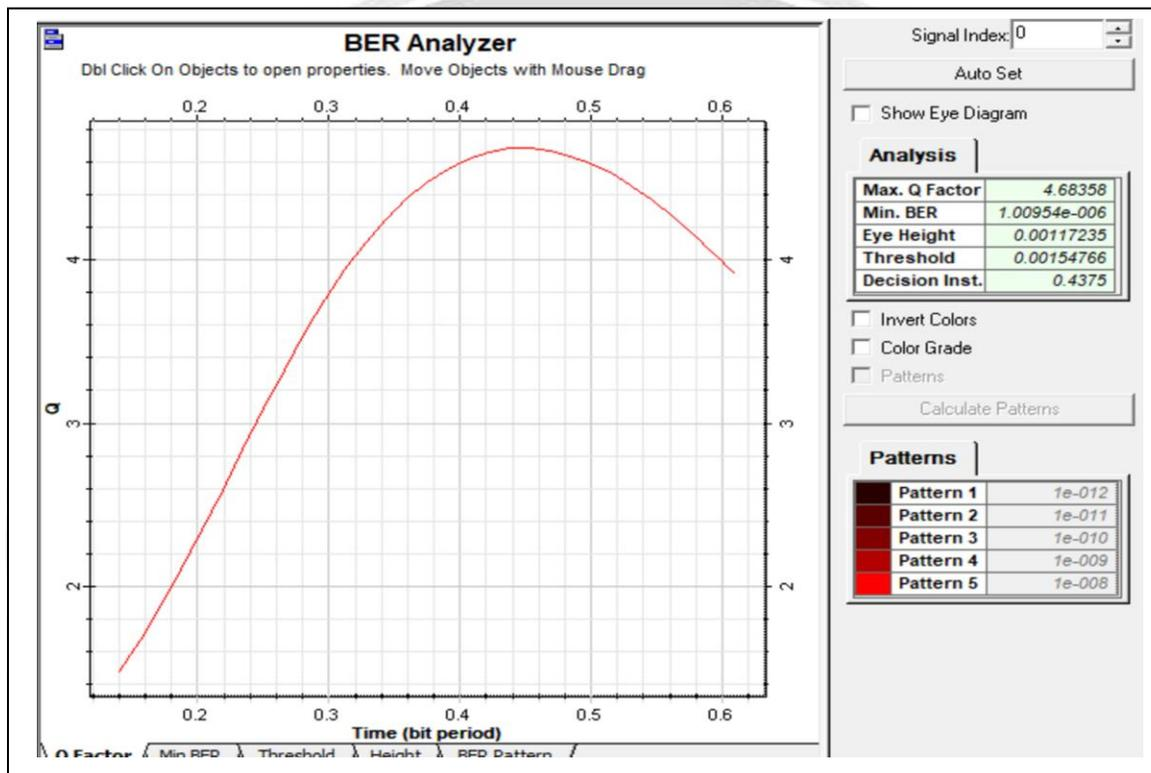
**Figure 5: BER and Q Factor Simulation Result at 1km with Rain.**
