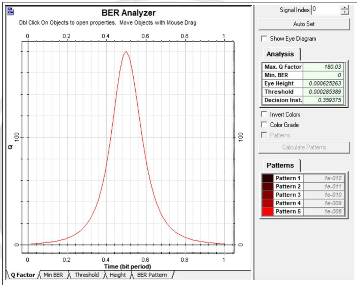
**Figure 6. BER and Q Factor Simulation Result at 100m with Fog.**
