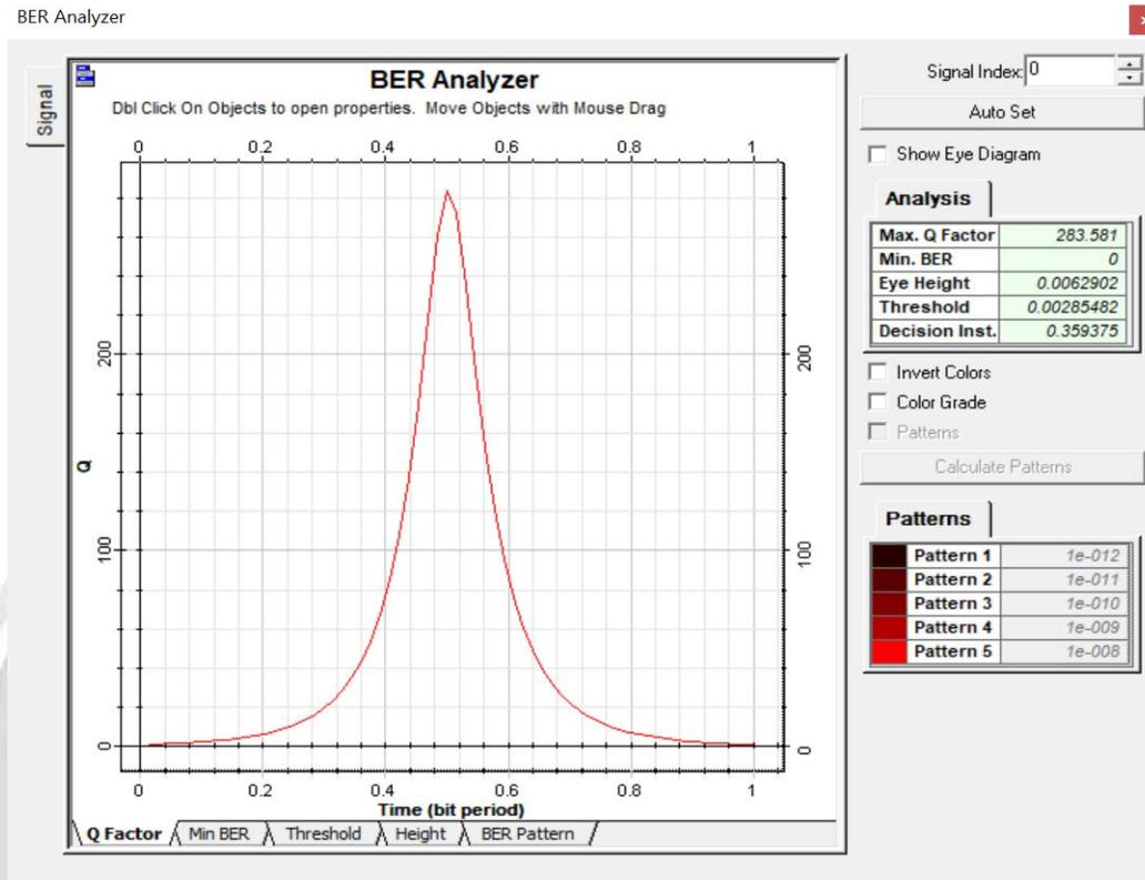
**Figure 4. BER and Q Factor Simulation Result at 100m with Rain.**
