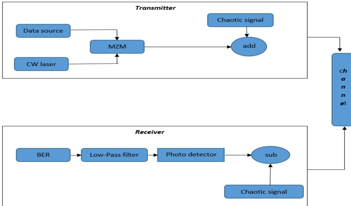
**Figure 2. Design communication circuit of VLC.**
