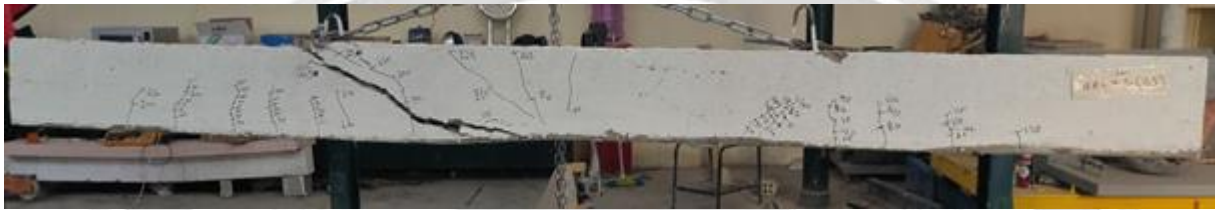
Fig (15) The crack pattern and mode of failure of specimen BR100TS1
