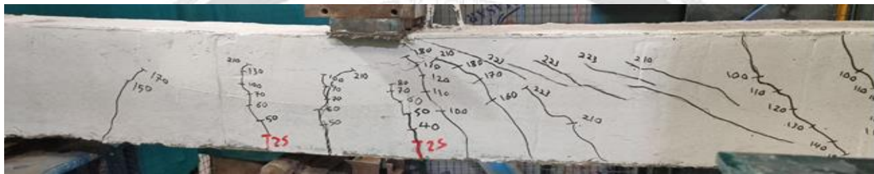
Fig (7) crack patterns and failure mode of specimen BROF1
