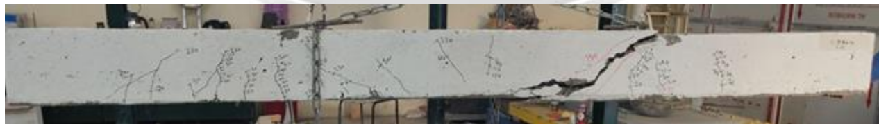
Fig (13) The crack pattern and mode of failure of specimen BR0S1
