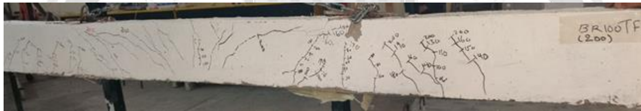
Fig (12) Crack patterns and failure mode of specimens BR100Tf
