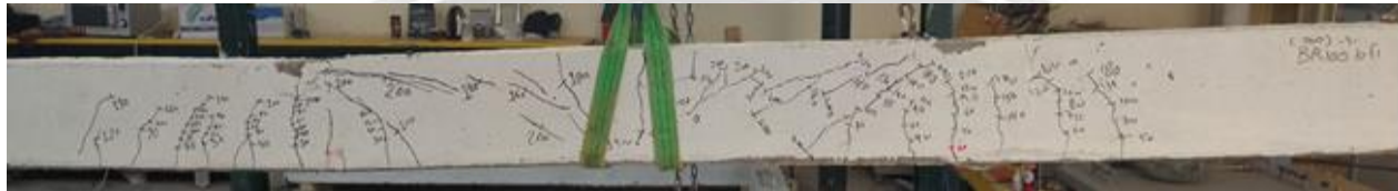
Fig (11) Crack patterns and failure mode of specimens BR100bf
