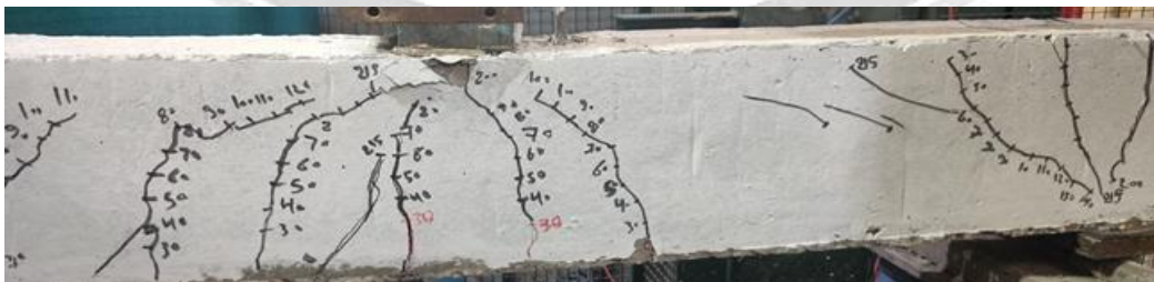
Fig (8) The failure mode and crack pattern for specimen BR20F1
