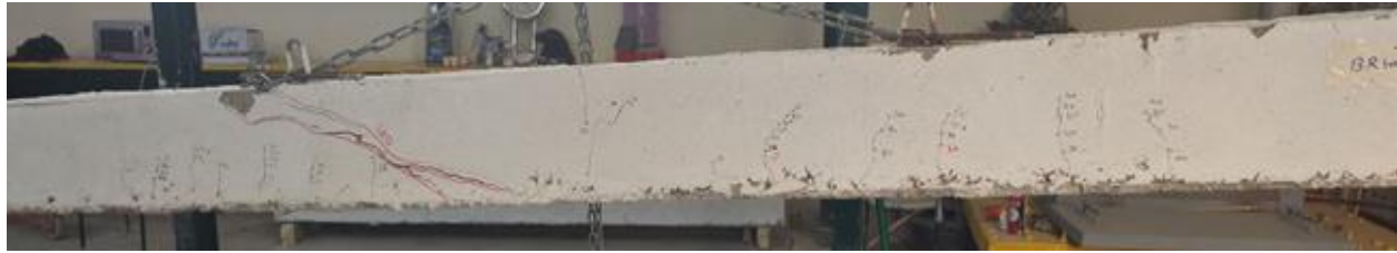
Fig (14) The crack pattern and mode of failure of specimen BR100bs1
