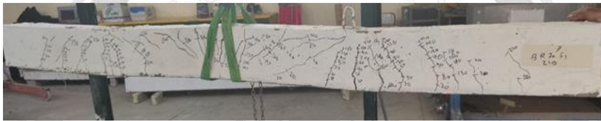
Fig (10) The failure mode and crack pattern for specimen BR40F
