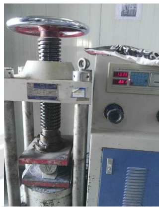
(b) Cylinder concrete under splitting strength.
