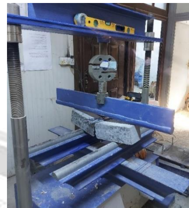
(c) Three-point load flexural test.
