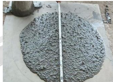
Fig. 8: T_{500} and Slump test for concrete mixture.
