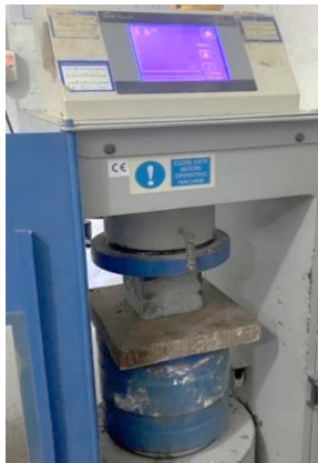
(a) Cubes concrete under compression.
