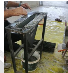
Fig. 9: V-funnel test apparatus.
