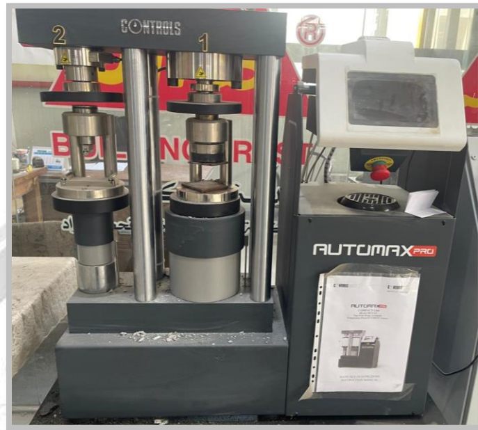
Figure 2. Compact-Line, 300 and 300/15 Kn. Top-of-the Rang Automatic, Compression-Flexural, Cement Tester.
