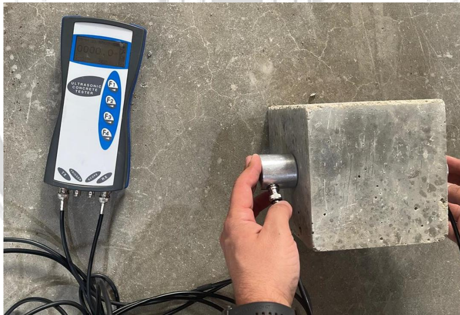
Figure8. shows ultrasonic concert tester. Ultrasonic pulse velocity (UPV) was performed at ages 7, 14, 28 and 56 days.
