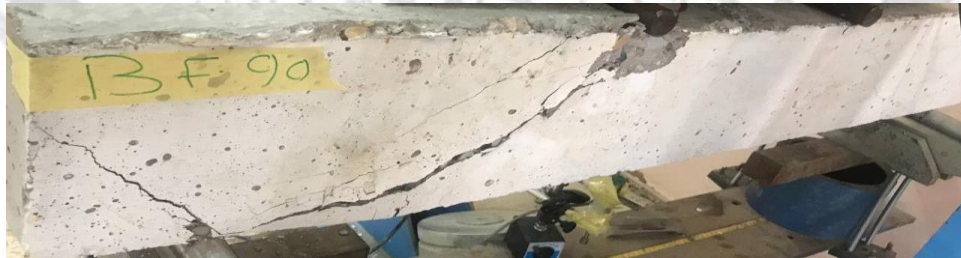
Fig. 5: Typical failure mode of control beam
