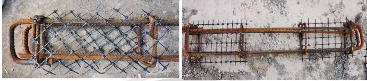
Fig. 4: Applying geogrid reinforcements to the steel cage
