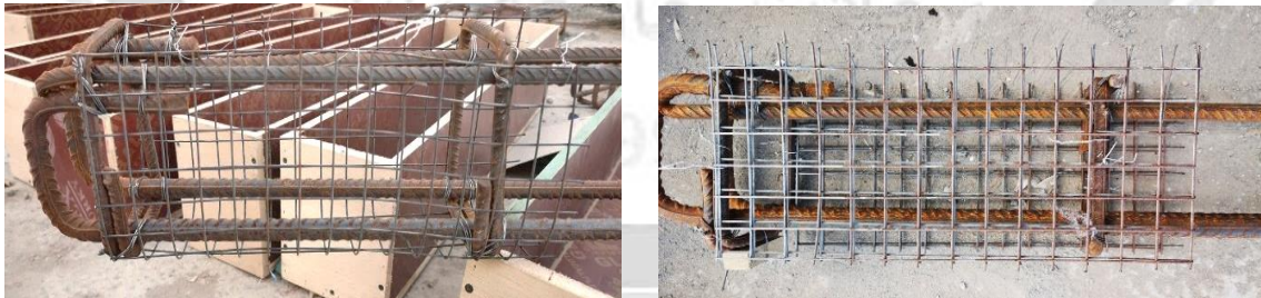
Fig. 2: Applying GFRP grid reinforcements to the steel cage
