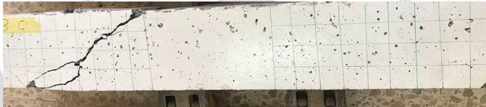
Fig. 5: Typical failure mode of control beam
