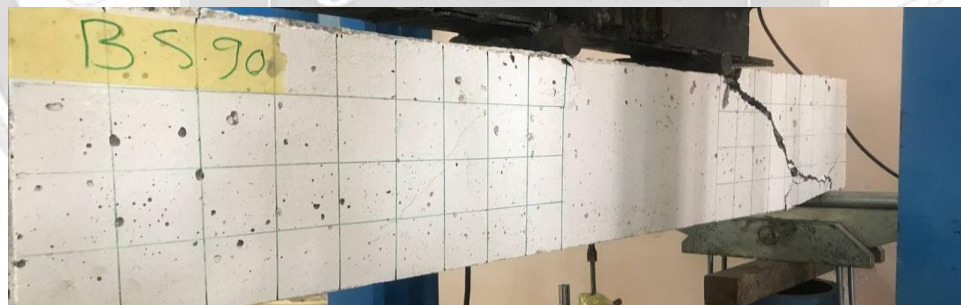
Fig. 6: Typical failure mode of beams strengthened by GFRP mesh
