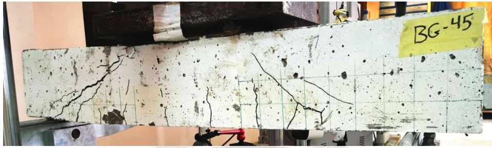
Fig. 8: Typical failure mode of beams strengthened by geogrid
