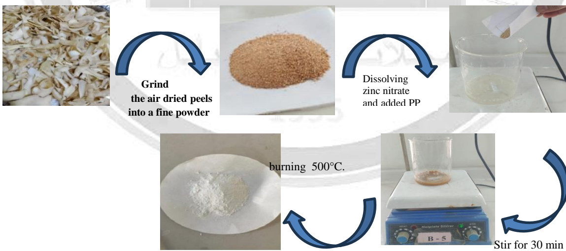
Fig. (1): ZnO-PP preparation steps.
