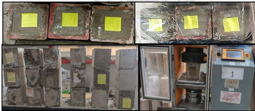
Figure (5) Compressive strength casting and Test (3 Cubes for each
