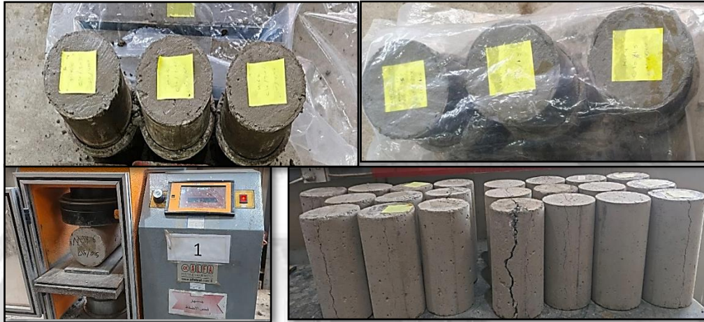
Figure (7) Test and Specimens casting of Split Tensile Strength (Three Cylinders for each Mix)
