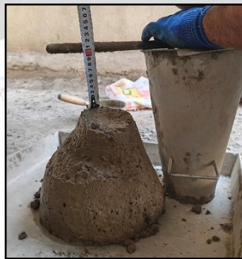
Figure (2) Slump Test.
