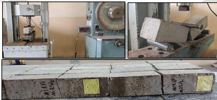
Figure (9) Modulus of Rupture Testing and Samples after Test.
